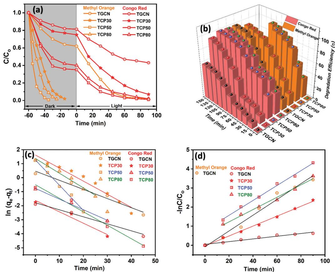
Fig. 2 (a)  $C/C_0$  vs. time (min), (b) degradation efficiency, (c) pseudo first-order rate kinetics of adsorption and (d) pseudo first-order rate kinetics of the photocatalytic degradation of MO and CR dyes using TGCN and TCP nanocomposites.
