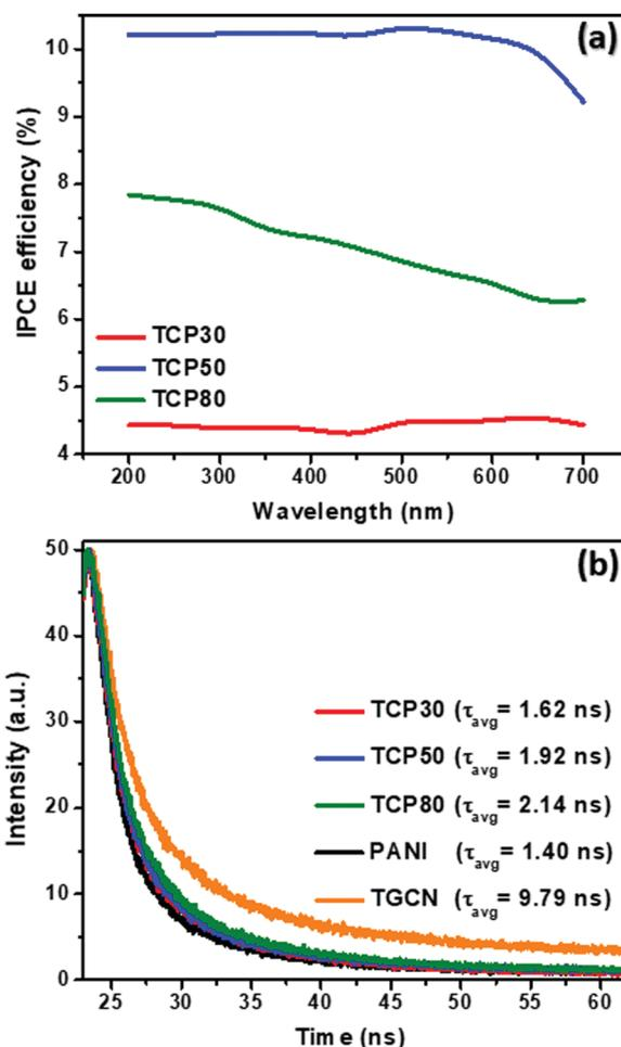
Fig. 4 (a) Comparison of the IPCE spectra as a function of the wavelength, (b) TRPL decay profile of the TGCN, PANI and TCP nanocomposites.
