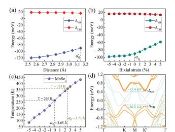
Fig. 4 (a and b) valley-splitting changes versus interlayer distance and biaxial strain, respectively. (c) Curie temperatures changes versus biaxial strain of monolayer MnSe<sub>2</sub>. (d) Band structure of MoTe<sub>2</sub>/MnSe<sub>2</sub> under 5% tensile strain
