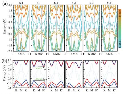
Fig. 2 (a) Band structure of the MoTe<sub>2</sub>/MnSe<sub>2</sub> heterobilayer in six stackings. The Fermi energy level is set to zero. (b) The corresponding enlarged details of valley splitting for the MoTe<sub>2</sub> monolayer. The red and blue lines denote the spin-up and spin-down bands, respectively, for the monolayer MoTe<sub>2</sub>.  $\Delta_{VB}$ and  $\Delta_{CB}$  are the valence- and conduction-band valley splittings, respectively
