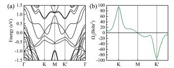
Fig. 3 (a and b) MLWF calculated band structure and the corresponding Berry curvature of the monolayer  $MoTe_2$  in the heterobilayer, respectively.
