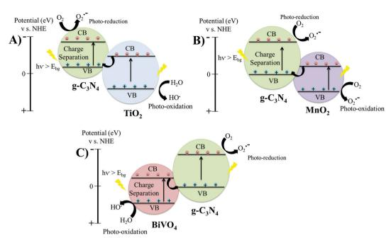
Fig. 6 Schematic of band structures and charge transfer mechanism in direct Z-scheme heterojunction structures: (A)  $g-C_3N_4-TiO_2$ ; (B)  $g-C_3N_4/MnO_2$ ; and (C)  $TBiVO_4/g-C_3N_4$ .
