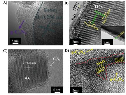
Fig. 5 TEM micrographs of (A) the type I  $FeS_2/g-C_3N_4$  heterojunction structure reprinted with permission from Elsevier; <sup>88</sup> (B) a type II  $TiO_2/ZnO$  heterojunction reprinted with permission from Nature; <sup>91</sup> (C) a direct Z-scheme  $g-C_3N_4-TiO_2$  heterojunction reprinted with permission from RSC<sup>96</sup> and (D) a direct Z-scheme  $g-C_3N_4/MnO_2$  reprinted with permission from ACS publications. <sup>98</sup>
