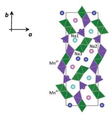
Fig. 1 The crystal structure of  $Na_{0.44}MnO_2$ , showing the ordering of  $Mn^{3+}$ (violet) and Mn<sup>4+</sup> (green) ions and the presence of three distinct crystallographic sites for Na (Na1 cyan, Na2 pink, and Na3 blue).
