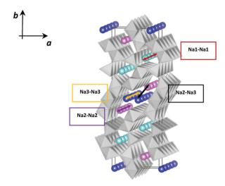
Fig. 2 Schematic representation of four possible Na<sup>+</sup> ion diffusion paths in Na<sub>0.44</sub>MnO<sub>2</sub>; Na1 cyan, Na2 pink, and Na3 blue.
