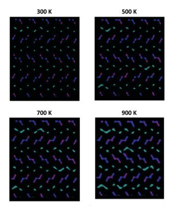
Fig. 8 Comparison among the Na<sup>+</sup> ion trajectories of Na<sub>0.44</sub>MnO<sub>2</sub> sample, with 71% of Na1 sites occupied, as the temperature changes: view along the c axis (see Fig. S4, ESI $\dagger$  – for a view along the a axis). For the sake of clarity, only the positions occupied by the Na<sup>+</sup> ions are reported; each point represents a position occupied by Na<sup>+</sup> along the simulation time. Legend: Na1 - cyan; Na2 - purple; Na3 - blue.
