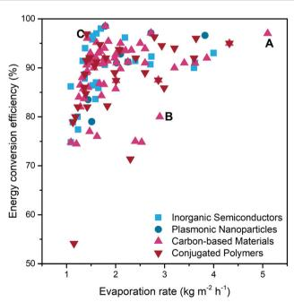
Fig. 14 The diagram summarises the solar water purification performance of different systems. Data acquired from ref. 24-27, 34-36, 42-45, 48-69, 73-130, 132-134, 137-153, 155-160, 162-167 and 169-184 (all the studies in this figure are under the solar intensity of 1 sun; studies with energy conversion efficiency >100% are not included for fair comparison).
