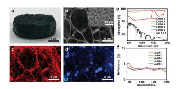
**Fig. 2** (a) Photo of the as-prepared  ${\rm Ti_2O_3}$ –PVA sponge-like hydrogel sample. (b) SEM image of the sponge-like hydrogel and EDS mapping of (c) carbon and (d) titanium. (e) Absorption and (f) reflectance spectra in the wavelength range of 200–2000 nm. Reproduced with permission.<sup>24</sup> Copyright 2019, American Chemical Society.
