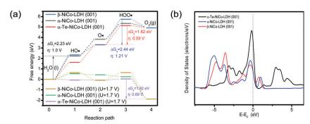
Fig. 8 DFT calculations of  $\alpha$ -NiCo-LDH,  $\beta$ -NiCo-LDH, and  $\alpha$ -Te-NiCo-LDH (001) surface for OER (a). And the total density of states analysis for these electrodes (b).
