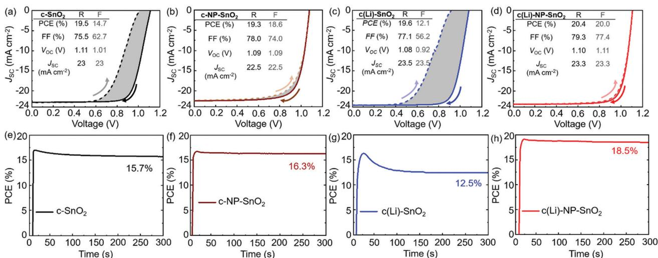
Fig. 2 Reverse (R) and forward (F) J-V scans and stabilized PCE (s-PCE) derived from MPP tracking of champion PSCs with (a and e) c-SnO<sub>2</sub>, (b and f) c-NP-SnO<sub>2</sub>, (c and g) c(Li)-SnO<sub>2</sub> and (d and h) c(Li)-NP-SnO<sub>2</sub> ETLs.
