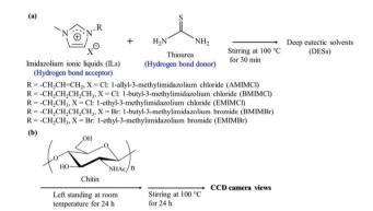
Fig. 3 (a) Preparation of DESs and (b) dissolution experiment procedure of chitin in DESs. 63 Copyright 2019 Multidisciplinary Digital Publishing Institute.
