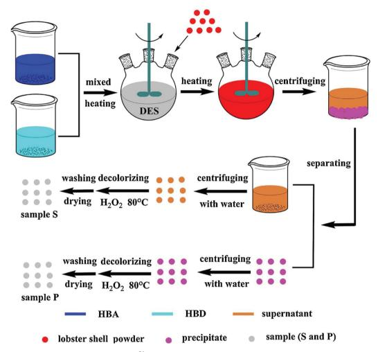
Fig. 4 Schematic diagram of the DES extraction process.<sup>64</sup> Copyright 2017 Elsevier Ltd.
