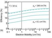
Fig. 5 (a) Simulated Efficiency as a function of absorption strength. Solid lines indicate a device thickness of 1 micrometer and dashed lines a thickness of 2 micrometers. (b) Simulated efficiency as a function of electron mobility for different hole mobilities (0.1–  $100 \text{ cm}^2 \text{ V}^{-1} \text{ s}^{-1}$ ). A carrier lifetime of 10 ns is assumed. The vertical grey line indicates the typical carrier mobility arising from grain boundary scattering.
