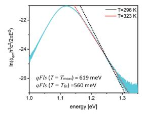
Fig. 2 Replotted PL flux to extract qFls from the fit to generalised Planck's law. The red line shows the fit with the temperature as a fit parameter, the black line shows the fit where the temperature has been fixed to the measurement temperature (296 K). The sample is a  $Cu(ln,Ga)Se_2$  film.
