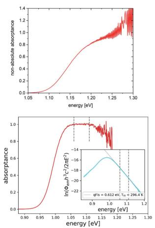
Fig. 6 Non-absolute absorptance spectra extracted from PL spectra using eqn (7). Top: from PL spectrum in Fig. 2, bottom: from sample #11 (replotted PL spectrum shown in the inset). Vertical lines indicate the fit range.
