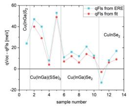
Fig. 4 Comparison for various chalcopyrite solar cells. (Top) difference between qFls determined by the two different methods. (Bottom) Comparison between  $V_{\rm OC}$  and qFls.
