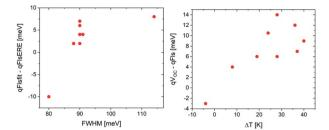
Fig. 5 Trends of the errors: discrepancy between the two methods to determine qFls as a function of the FWHM of the PL peak and the discrepancy between  $V_{\rm OC}$  and qFls from the fit to generalised Planck's law as a function of the discrepancy between the fitted temperature and the measurement temperature.
