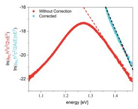
Fig. 3 (Top) Non-absolute absorptance extracted from the PL spectrum in the inset. (Bottom) Replotted PL spectra for the fit to generalised Planck's law, original (red) and divided by the separately measured absorptance spectrum (light blue). The fitting range is in both cases from 1.42 eV to 1.47 eV. The sample is a methylammonium Sn iodide film.
