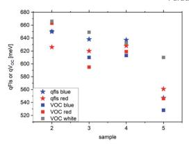
Fig. 7 gFls and  $V_{OC}$  for the Cu(In,Ga)(S,Se)<sub>2</sub> samples illuminated with a red laser (660 nm), a blue laser (405 nm) or a simulated AM1.5 spectrum (white).
