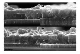
Fig. 5 Cross-section of devices with absorber thickness of about 250 nm. (a) No passivation layer and no NaF. (b) No passivation layer and NaF deposited onto CZTS precursor before annealing. (c)  $Al_2O_3$  passivation and NaF deposited onto CZTS precursor prior to annealing. (d)  $HfO_2$  passivation layer and NaF deposited onto CZTS precursor prior to annealing.
