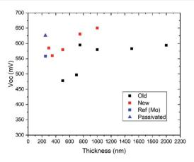
Fig. 1  $V_{\rm OC}$  as a function of absorber thickness comparing published data (black) and new data (red), all on Mo back contact. Two devices (blue) from a different series using 250 nm thick CZTS comparing Mo and Mo/Al<sub>2</sub>O<sub>3</sub> back contact are also shown (see Table 2).
