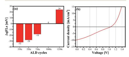
Fig. 4 (a) Bar chart showing the change in the qFLs of  $Cu(In,Ga)S_2$  absorber before and after buffer deposition as a function of the (Zn,Sn)O buffer thickness. (b) The characteristic J-V curve of the  $Cu(In,Ga)S_2$  device prepared with a50 nm thick (Zn,Sn)O buffer layer deposited at 120 °C.
