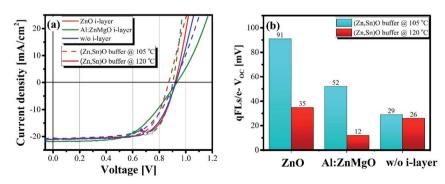
Fig. 2 (a) The characteristic J-V curves of the Cu(In,Ga)S<sub>2</sub> devices prepared with (Zn,Sn)O buffer layers deposited at 105 °C (B1) and 120 °C (B2), represented by dashed and solid lines respectively. The devices prepared with ZnO, Al:ZnMgO and without an i-layer are represented by red, green and blue lines, respectively. (b) Interface  $V_{\rm OC}$  deficit bar plot of devices made with B1 and B2 with various i-layer combinations.
