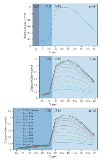
Fig. 6 The 2D sensitivity analysis was performed with the updated simulation reference to evaluate the effects of changing the barrier height at the CdS contact along S1 (a), S2 (b), and S3 (c). The legend displayed in panel (c) refers to all panels. All curves overlap in panel (a).
