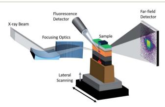
Fig. 2 Schematic of the experimental setup. Incoming X-rays are focused using KB mirrors down to  $80 \text{ nm} \times 80 \text{ nm}$ . The sample is raster-scanned in the lateral plane. A far-field detector measures the diffraction signal of the transmitted beam, and an energy-dispersive fluorescence detector collects fluorescence photons. The X-ray beam induced current in the semiconductor device is amplified and measured at every scan position.
