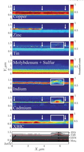
Fig. 3 XRF images of the main elements constituting the sample together with the XBIC signal, resulting in the specification of the layered structure with the computational domain between red lines. The white arrows highlight the areas associated with composition variations in the CZTS layer and the white box indicates the area with an inhomogeneous distribution of elements from the CdS and ITO layers, as well as the absence of the ZnO layer.
