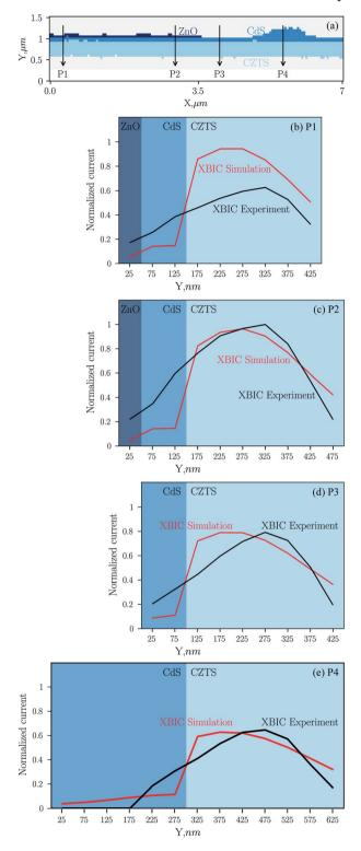
Fig. 7 The computational domain (a) with the location of line profiles from the experimental and simulated data along P1, P2, P3 and P4 shown in (b-e).
