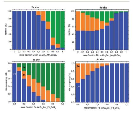
Fig. 7 Comparison of the cation distribution in the  $Cu_2(Zn_xMn_{1-x})SnSe_4$  (above) and  $Cu_2(Zn_xMn_{1-x})SnSe_4$  (below) solid solution series. For simplicity, the 2c and 2d sites of the kesterite type structure are transformed into the equivalent 4d site of the stannite type structure (right figures). The cation distribution on the 2a sites of the kesterite and stannite type structures are shown in the left figures.
