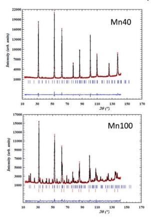
Fig. 4 Rietveld refinement of the neutron diffraction data for  $Cu_{2.01}Zn_{0.62}Mn_{0.42}Sn_{0.98}Se_4$  (left) and  $Cu_{2.05}Mn_{0.98}Sn_{0.99}Se_4$  (right). The red dots are experimental data, the black line is the obtained fit, the blue ticks are the Bragg peak positions of the kesterite and stannite type structures, respectively, the red ticks are the Bragg peak positions of the MnSe phase, and the blue line is the difference between the experimental and calculated data.
