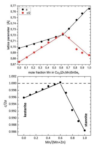
Fig. 3 Lattice parameters a and c (top) and tetragonal distortion c/2a (bottom) of Cu<sub>2</sub>(-Zn<sub>x</sub>Mn<sub>1-x</sub>)SnSe<sub>4</sub> mixed crystals depending on the chemical composition. The lines are guides for the eye.
