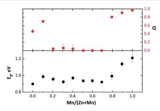
Fig. 9 Band gap energy  $E_{\rm g}$  and order parameter Q of  ${\rm Cu_2(Zn_{1-x}Mn_x)SnSe_4}$  mixed crystals dependent on the Mn/(Mn + Zn) ratio.
