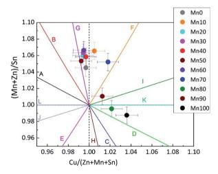
Fig. 2 Cation ratio plot showing the  $Cu_2(Zn_{1-x}Mn_x)SnSe_4$  mixed crystals synthesized. All of the Zn-rich mixed crystals are located between the G and F type lines. The Mn-rich  $Cu_2(Zn_{1-x}Mn_x)SnSe_4$  mixed crystals show a wider spread over the Cu-rich,  $B^{II}$ -rich area of the cation ratio plot. Each point refers to a homogeneous, single phase quaternary phase. The off-stoichiometry types refer to Table 4 and ref. 12.
