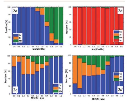
Fig. 6 Cation distribution model for the end members Cu<sub>2</sub>ZnSnSe<sub>4</sub> and Cu<sub>2</sub>MnSnSe<sub>4</sub>, as well as the  $Cu_2(Zn_xMn_{1-x})SnSe_4$  mixed crystals, as determined experimentally by neutron diffraction. The cation sites 2a, 2b, 2c and 2d of the kesterite type structure are shown.
