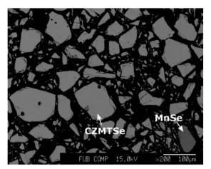
Fig. 1 BSE micrograph of the  $Cu_2(Zn_{1-x}Mn_x)SnSe_4$  sample with x=0.9. Grains of the quaternary phase, with the chemical composition  $Cu_{2.02}Zn_{0.10}Mn_{0.90}Sn_{0.99}Se_4$ , as well as grains of the secondary phase are visible (gray grains). The black part of the image is the epoxy in which the grains are embedded.
