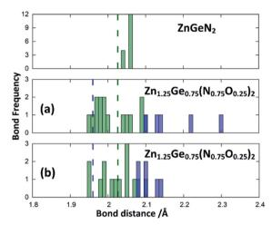
Fig. 4 Zn-N (green) and Zn-O (blue) distances from the structure optimisations of the crystal structures for  $ZnGeN_2$  (top) and the two configurations of  $Zn_{1.25}Ge_{0.75}(N_{0.75}O_{0.25})_2$ , as depicted in Fig. 2. The expected distances from the bond valences are given as dashed lines.
