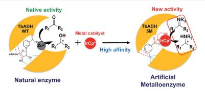
Fig. 1 Schematic representation of the design of ArMs: left, the natural catalysis in TbADH WT involving NADP<sup>+</sup> and a catalytic Zn<sup>2+</sup>; right, the supramolecular insertion of an iridium piano stool complex (red) inside the NADP+ cofactor pocket and Zn2+ binding region of TbADH 5M with high affinity induced by the anchor substructure (R).
