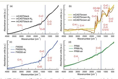
Fig. 5 Vector normalized ATR-AB (Attenuated Total Reflection-Absorption) spectra from FTIR measurements for fresh, oven-air ( $N_2 + O_2$ )- and  $-N_2$ -heated soot. Likely chemical bond assignments are indicated in the individual spectra. The blue line corresponds to the wavenumber 1330 cm<sup>-1</sup> which separates the characteristic (left) and the fingerprint region (right).
