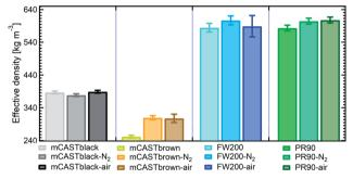
Fig. 18 The effective density ( $\rho_{\rm eff}$ ) of fresh and denuded 200 nm soot particles. The error bar indicates one standard deviation. Please note the y-axis origin.
