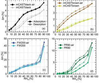
Fig. 7 Dynamic water vapour sorption (DVS) isotherms for fresh and synthetic air  $(N_2 + O_2)$  oven-heated (300 °C) soot. The solid lines with closed symbols and dashed lines with open symbols indicate adsorption and desorption isotherms, respectively. Each isotherm loop represents for an individual measurement. Note different y-axis scales.
