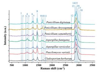
Fig. 2 Single-particle Raman spectra of seven different fungus samples optically trapped in a reaction chamber under controlled environment.
