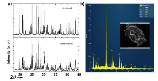
Fig. 2 (a) X-ray diffraction pattern of Ba<sub>5</sub>Fe<sub>2</sub>In<sub>4</sub>ZnS<sub>15</sub> calculated from single crystal refinement, and compared to the X-ray experimental pattern of the obtained powder; impurity peaks are indexed to blue circles. (b) EDX analysis with atomic ratios and SEM image of a crystal (inset).
