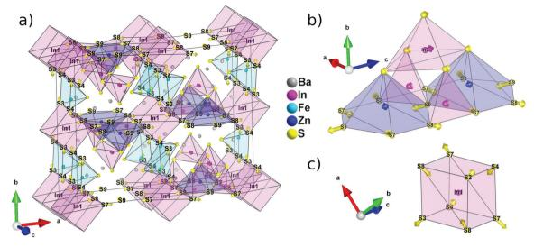
Fig. 3 Representation of the centrosymmetric (Amam) hypothetical aristotype of Ba<sub>5</sub>ZnFe<sub>2</sub>In<sub>4</sub>ZnS<sub>15</sub> and the atomic shifts necessary to derive the real structure. The arrows representing the atomic displacements are drawn to scale meaning that the tip of the arrows points to the real position of the atoms. The position identification refers to the Ama2 cell. (a) Whole cell, (b) T2 super-tetrahedral subunit and (c) coordination sphere of In1.
