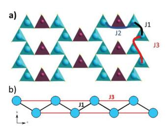
Fig. 5 (a) Magnetic exchange coupling scheme of J1, J2 and J3 between iron atoms. (b) Quasi one-dimensional zigzag magnetic chain built from iron atoms in blue with J1 and J3 intra-chain magnetic exchanges represented in black and red, respectively.
