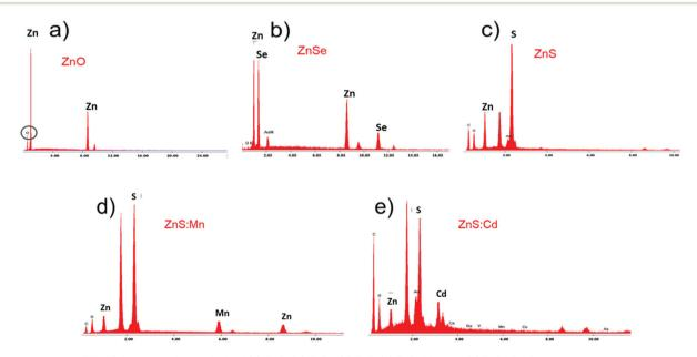
Fig. 3 X-ray spectra (EDAX) for qualitative analysis of (a) ZnO, (b) ZnSe, (c) ZnS, (d) ZnS: Mn, and (e) ZnS: Cd Qds
