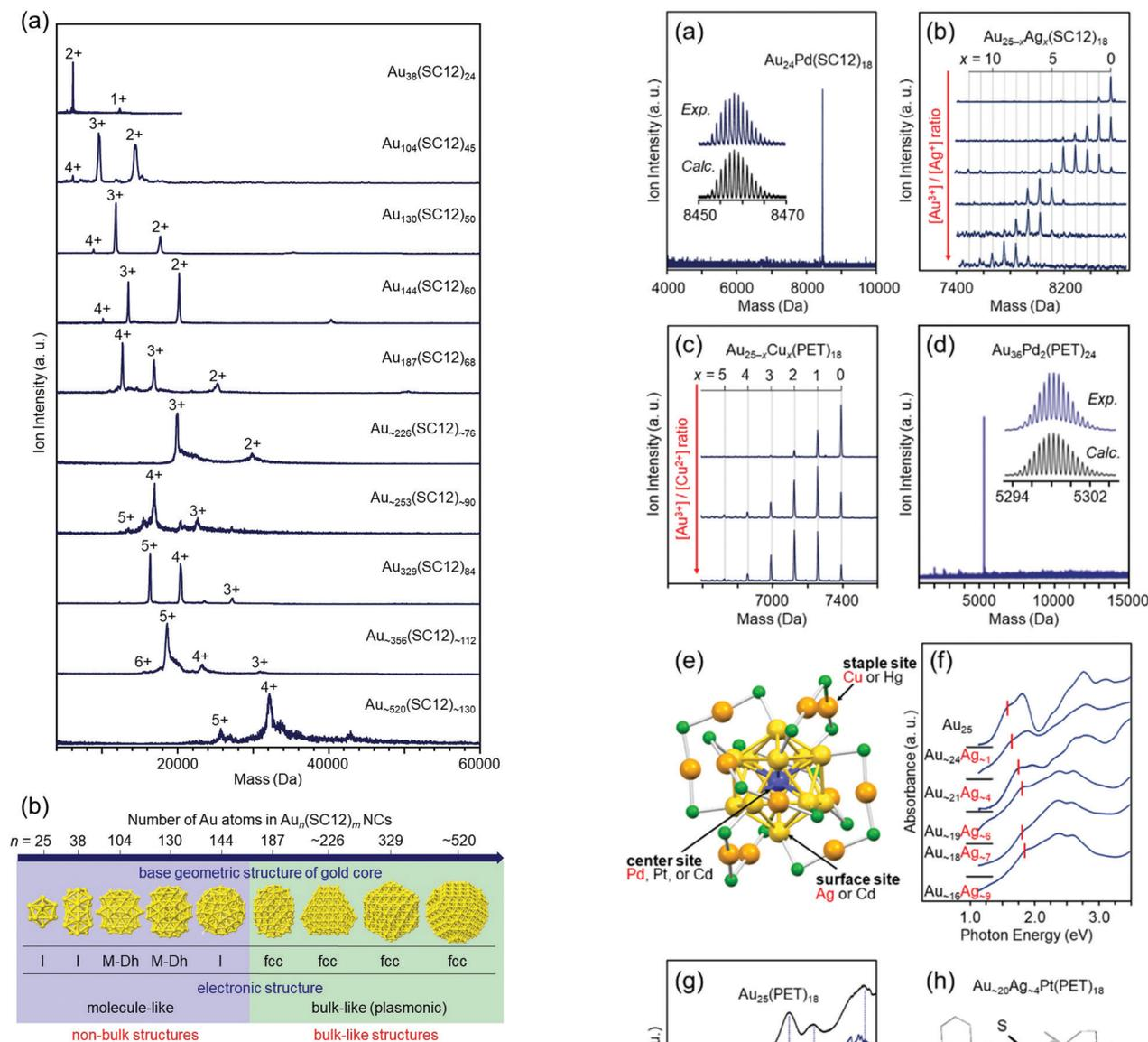
Fig. 5 (a) Positive-ion ESI mass spectra of  $Au_n(SC12)_m$  NCs. (b) Non-bulk to bulk transition between  $Au_{144}(SC12)_{60}$  and  $Au_{187}(SC12)_{68}$  in the  $Au_n(SC12)_m$ -NC system.<sup>109</sup> Reproduced with permission from ref. 109. Copyright 2015 American Chemical Society.
