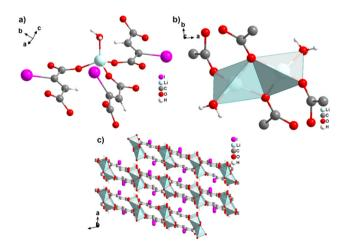
Fig. 42 Crystal structure of [Li(HOOC-CH=CI-COO)(H<sub>2</sub>O)] showing: (a) the coordination sphere of the Li+ cation, (b) the dinuclear building unit, and (c) stacked two-dimensional layers. Graphics redrawn from the cif file (CSD-Refcode WAVXEX).132
