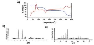
Fig. 20 (a) Thermogravimetric (blue trace) and DTA curves (red trace) of [Cd(ADC)(H<sub>2</sub>O)<sub>3</sub>]·H<sub>2</sub>O, (b) and (c) powder X-ray diffraction patterns of [Cd(ADC)(H<sub>2</sub>O)<sub>3</sub>]·H<sub>2</sub>O and [Cd(ADC)(H<sub>2</sub>O)<sub>2</sub><sub>3</sub>], respectively. Reproduced from ref. 60 with permission of American Chemical Society, copyright 2003.
