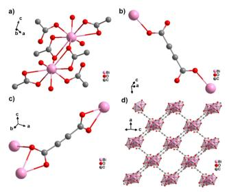
Fig. 25 Crystal structure of bismuth acetylenedicarboxylate [Bi(ADC)<sub>1.5</sub>(H<sub>2</sub>O)<sub>2</sub>]·2H<sub>2</sub>O showing: (a) the coordination environment of two Bi3+ cations, (b) and (c) the coordination mode of two crystallographically different ADC linkers, and (d) the resulting 2D layer by connecting dinuclear {Bi<sub>2</sub>O<sub>8</sub>(H<sub>2</sub>O)<sub>6</sub>} units with ADC linkers. Graphics redrawn from the cif file (CSD-Refcode NERQOS).67
