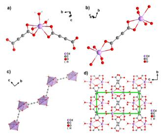
cadmium Fig. 19 Crystal structure of acetylenedicarboxylate [Cd(ADC)(H<sub>2</sub>O)<sub>3</sub>]·H<sub>2</sub>O showing: (a) the coordination environment of the Cd<sup>2+</sup> cation, (b) the coordination mode of the ADC linker, (c) the onedimensional zigzag chain, and (d) the packing of the framework viewed along [100], showing chains held together by hydrogen bonds (not emphasized). Graphics redrawn from the cif file (CSD-Refcode MUGJED). 59
