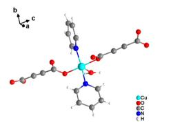
Fig. 16 Cu<sup>2+</sup> coordination sphere in the crystal structure of [Cu(ADC)(Py)<sub>2</sub>(H<sub>2</sub>O)]. Graphics redrawn from the cif file (CSD-Refcode KIVPEV).56
