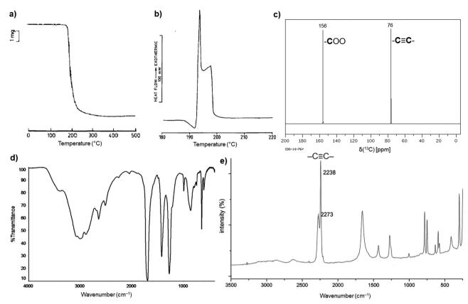
Fig. 1 (a) Thermogravimetric curve under air, (b) differential scanning calorimetry (DSC) curve, (c) <sup>13</sup>C NMR spectrum in D<sub>2</sub>O, (d) FT-IR spectrum and (e) Raman spectrum of H<sub>2</sub>ADC. Adapted from ref. 30-33 with permission of Elsevier, copyright 1987; copyright 2014 and permission of John Wiley & Sons, copyright 2021.
