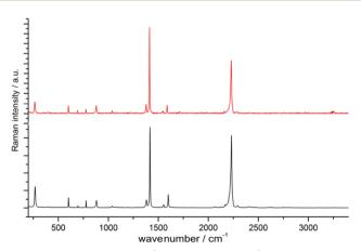
Fig. 11 Raman spectra of [Eu<sup>II</sup>(ADC)] (red) and [Sr<sup>II</sup>(ADC)] (black), both displaying the strong bands of -C≡C-stretching vibrations of ADC at  $\sim$  2250 cm<sup>-1</sup>. Reproduced from ref. 50 with permission of Wiley & Sons, copyright 2020.
