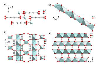
Fig. 4 Crystal structure of anhydrous lithium acetylenedicarboxylate [Li<sub>2</sub>(ADC)] showing: (a) the coordination environment of the Li atom, (b) the chains of infinite edge-sharing LiO<sub>4</sub> tetrahedra, (c) the coordination mode of ADC connecting the alternatively perpendicular chains and (d) the three-dimensional packing of the framework viewed along the [100] direction. Graphics redrawn from the cif file (CSD-Refcode ICUHIA).41
