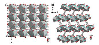
Fig. 31 Crystal structure of MIL-95 showing: (a) the packing of edge and corner-sharing EuO<sub>9</sub> polyhedra in the (010) plane and (b) the threedimensional packing of the framework. The crystal water molecules in the pores are omitted for clarity. Graphics redrawn from the cif file (CSD-Refcode FIFPOA).86
