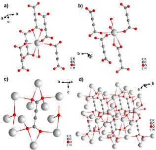
Fig. 6 Crystal structure of hydrated potassium acetylenedicarboxylate [K<sub>2</sub>(ADC)(H<sub>2</sub>O)] showing: (a) and (b) the coordination environment of the two crystallographically distinct K atoms, (c) the coordination mode of the ADC linker and water molecules, and (d) the complex three-dimensional framework structure. Graphics redrawn from the cif file (CSD-Refcode XADRUQ).42
