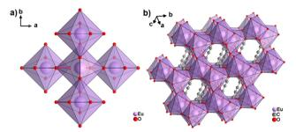
Fig. 10 (a) M<sup>II</sup>O<sub>8</sub> polyhedra and four edge-sharing neighbouring analogues, and (b) the three-dimensional packing of polyhedra and linkers found in the structure of ADC-based CPs with the formula [MII(ADC)], exemplified here by [EuII(ADC)]. Graphics redrawn from the cif file (CSD-Refcode IHUCUM).50
