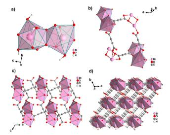
Fig. 29 Crystal structure of  $[Bi(ADC)_{1.5}(H_2O)_3]\cdot H_2O$  showing: (a) the dinuclear unit of two edge-sharing BiO<sub>8</sub> polyhedra, (b) the connectivity of ADC linkers, (c) the connection of the dimeric units in a view along [010] and (d) the three-dimensional packing of the framework. Non-coordinating water molecules within the pores are omitted for clarity. Graphics redrawn from the cif file (CSD-Refcode NERQUY).67
