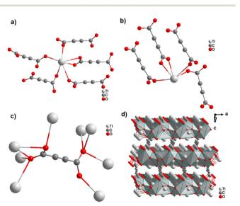
Fig. 21 Crystal structure of anhydrous thallium acetylenedicarboxylate [Tl<sub>2</sub>(ADC)] showing: (a) and (b) the coordination environment of two crystallographically distinct Tl+ cations, (c) the coordination mode of the ADC linker, and (d) the three-dimensional packing of the framework. Graphics redrawn from the cif file (CSD-Refcode TILFUQ01).<sup>61</sup>
