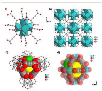
Fig. 32 Crystal structure of Zr-HHU-1 showing: (a) the hexanuclear Zr<sub>6</sub>cluster connected to twelve ADC linkers, (b) the three-dimensional packing of the fcu network, (c) the tetrahedral cavity, and (d) the octahedral cavity both with their available pores (yellow spheres) and triangular windows (green spheres). Graphics adapted from ref. 90 with permission of Wiley &
