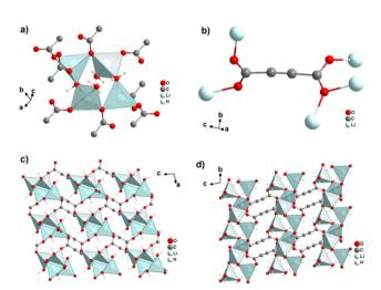
Fig. 3 Crystal structure of hydrated lithium acetylenedicarboxylate [Li<sub>2</sub>(ADC)(H<sub>2</sub>O)<sub>2</sub>] showing: (a) the tetranuclear ring unit of corner-sharing LiO<sub>4</sub> tetrahedra, (b) the coordination mode of the ADC linker and (c) and (d) the three-dimensional packing of the framework viewed along the [010] and [100] directions, respectively. Graphics redrawn from the cif file (CSD-Refcode ICUDOC).41
