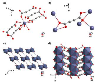
Fig. 24 Crystal structure of lead acetylenedicarboxylate [Pb(ADC)(H<sub>2</sub>O)] showing: (a) the coordination environment of a Pb2+ cation, (b) the coordination mode of the ADC linker, and (c) and (d) the packing of the crystal structure viewed along the [010] and [100] directions, respectively. Graphics redrawn from the cif file (CSD-Refcode MUZKEY).66
