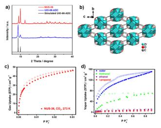
Fig. 33 (a) Powder X-ray diffraction pattern of NUS-36 compared with that of UiO-66-ADC, (b) three-dimensional packing of the bcu network of NUS-36, (c) CO<sub>2</sub> adsorption isotherm for NUS-36 at 273 K, and (d) adsorption isotherms of water, methanol, ethanol and i-propanol for NUS-36 at 273 K. Adapted from ref. 92 with permission of American Chemical Society, copyright 2019.
