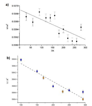
Fig. 38 Variation of unit cell volume with temperature for (a) [Sr(ADC)] and (b) [Eu<sup>II</sup>(ADC)]. Reproduced from ref. 44 with permission of John Wilev & Sons, copyright 2002, and from ref. 50 with permission of John Wiley & Sons, copyright 2020
