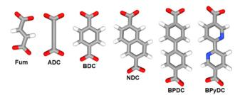
Scheme 1 Some linear dicarboxylate linkers used in the construction of CPs and MOFs. Each of these linkers has a doubly-negative charge. Better designations would be Fum<sup>2-</sup>, ADC<sup>2-</sup>, etc. For better readability we omit the charge in the text.
