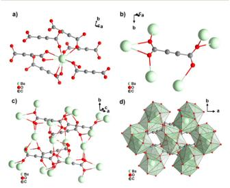
Fig. 9 Crystal structure of hydrated barium acetylenedicarboxylate [Ba(ADC)(H<sub>2</sub>O)] showing: (a) the coordination environment of the Ba atom, (b) the coordination mode of the ADC linker and (c) and (d) the threedimensional packing of the framework and the net of edge-sharing polyhedra, respectively. Graphics redrawn from the cif file (CSD-Refcode KIYJOR).39
