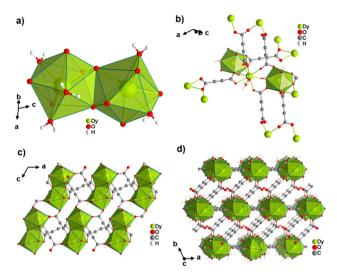
Fig. 30 Crystal structure of [Dy<sub>2</sub>(ADC)<sub>3</sub>(H<sub>2</sub>O)<sub>6</sub>]·2H<sub>2</sub>O showing: (a) the dinuclear unit of two edge-sharing DyO9 polyhedra, (b) the connectivity of ADC linkers, (c) the connection of the dimeric units in a view along [010] and (d) the three-dimensional packing of the framework. Non-coordinating water molecules within the pores are omitted for clarity. Graphics redrawn from the cif file (CSD-Refcode NILSUZ).85
