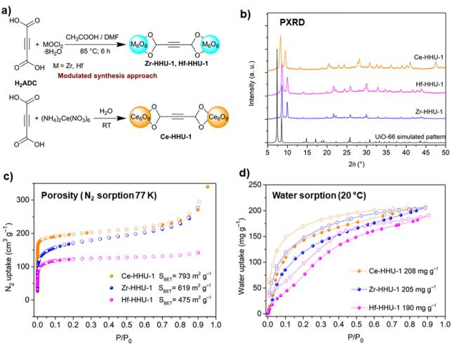
Fig. 34 (a) Reaction schemes for the synthesis of M-HHU-1 (M = Zr, Hf, Ce), (b) powder X-ray diffraction patterns of M-HHU-1 (M = Zr, Hf, Ce), compared with the simulated pattern for UiO-66, (c) nitrogen adsorption isotherms at 77 K, and (d) water sorption isotherms of M-HHU-1 (M = Zr, Hf, Ce) at 20 °C. Graphics adapted from ref. 34, 90 and 94
