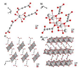
Fig. 5 Crystal structure of hydrated sodium acetylenedicarboxylate  $[Na_2(ADC)(H_2O)_4]$  showing: (a) the coordination environment of the Na atom, (b) the coordination mode of ADC linkers and water oxygen atoms, and (c) and (d) sheets from chains of NaO<sub>6</sub> octahedra connected by ADC linkers. Graphics redrawn from the cif file (CSD-Refcode XADSAX).42
