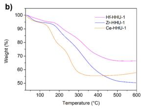
Fig. 35 (a) CO<sub>2</sub> adsorption isotherms of Ce-HHU-1 at 273 K and 293 K, and (b) thermogravimetric analyses of M-HHU-1 (M = Zr, Hf, and Ce). Graphics adapted from ref. 34, 90 and 94.
