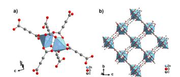
Fig. 27 Crystal structure of ZnADC1, (HHUN)<sub>2</sub>[Zn<sub>2</sub>(ADC)<sub>3</sub>]·(HHUN)(NO<sub>3</sub>), showing: (a) the dinuclear Zn<sub>2</sub> paddle-wheel unit connected by six ADC linkers and (b) the three-dimensional packing of the wine-rack-like framework. The HHUN+ cations and the (HHUN)(NO3) ionic pairs occupying the pores of the MOF framework are omitted for clarity. Graphics redrawn from the cif file (CSD-Refcode PAGRUO).58
