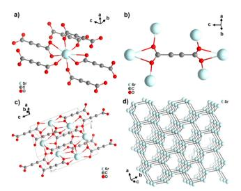
Fig. 8 Crystal structure of anhydrous strontium acetylenedicarboxylate [Sr(ADC)] showing: (a) the coordination environment of the Sr atom, (b) the coordination mode of the ADC linker, (c) the three-dimensional packing of the framework, and (d) the diamond-like arrangement of the strontium atoms. Graphics redrawn from the cif file (CSD-Refcode XUKKET01).44
