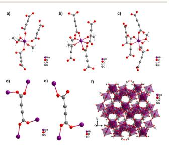
Fig. 18 Crystal structure of the non-porous 3D CP [Mn<sub>2</sub>(ADC)<sub>2</sub>(MeOH)<sub>5</sub>]: (a-c) coordination sphere of three crystallographically distinct Mn<sup>2</sup> cations, (d) and (e) coordination modes of two crystallographically distinct ADC linkers, and (f) structure packing viewed along [001]. Graphics redrawn from the cif file (CSD-Refcode PAGRAU).58
