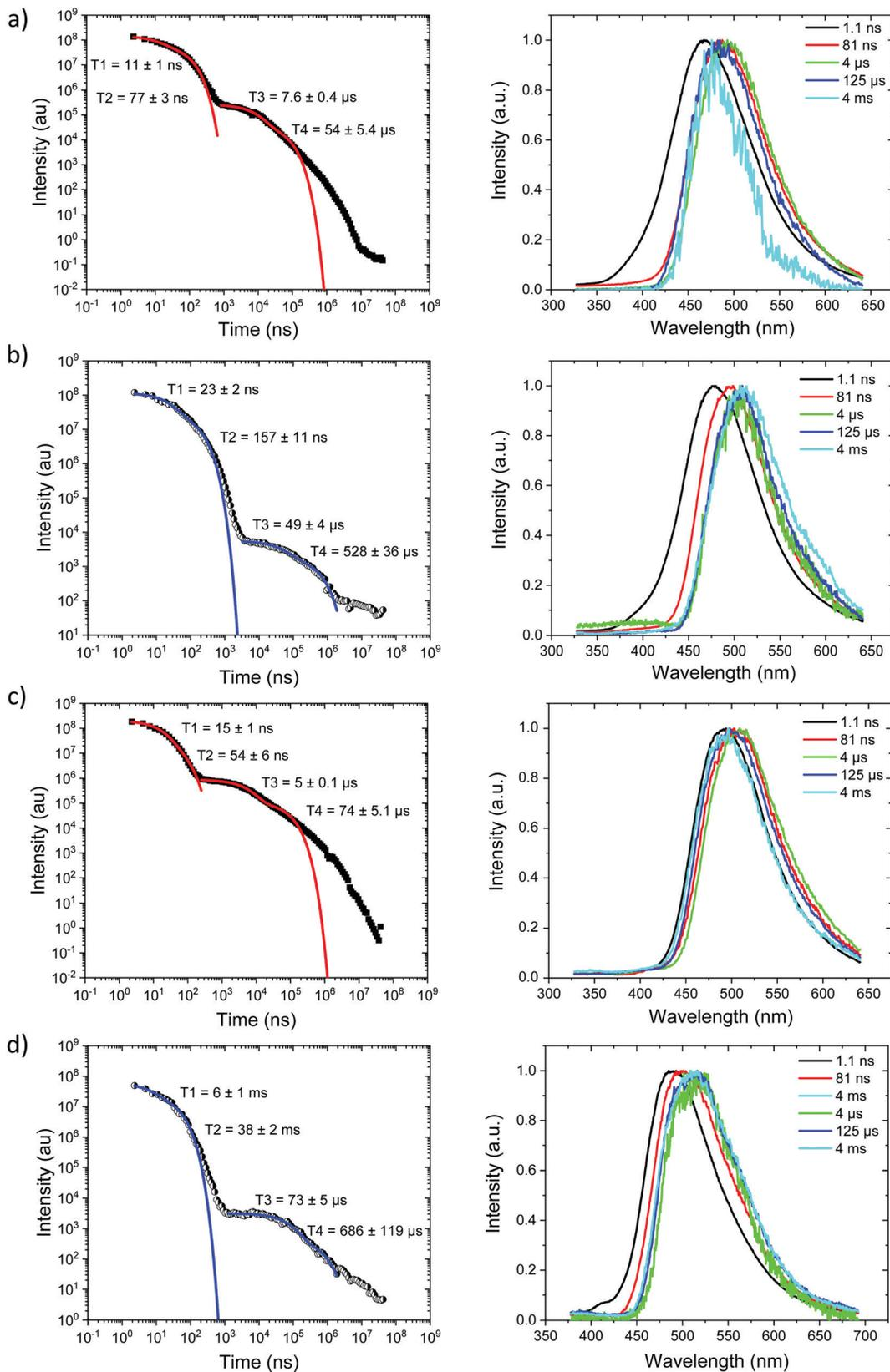
Fig. 4 Time-resolved spectrally integrated intensity decay (left) and representative time resolved spectra (right) of  $\text{Ph}_3\text{TRZCzTPA}$  (a) 300 K and (b) 80 K;  $\text{Ph}_2\text{TRZCzTPA}$  (c) 300 K and, (d) 80 K in zeonex matrix. Spectral times given in ns, and decay fitting data included in the decay plots.
