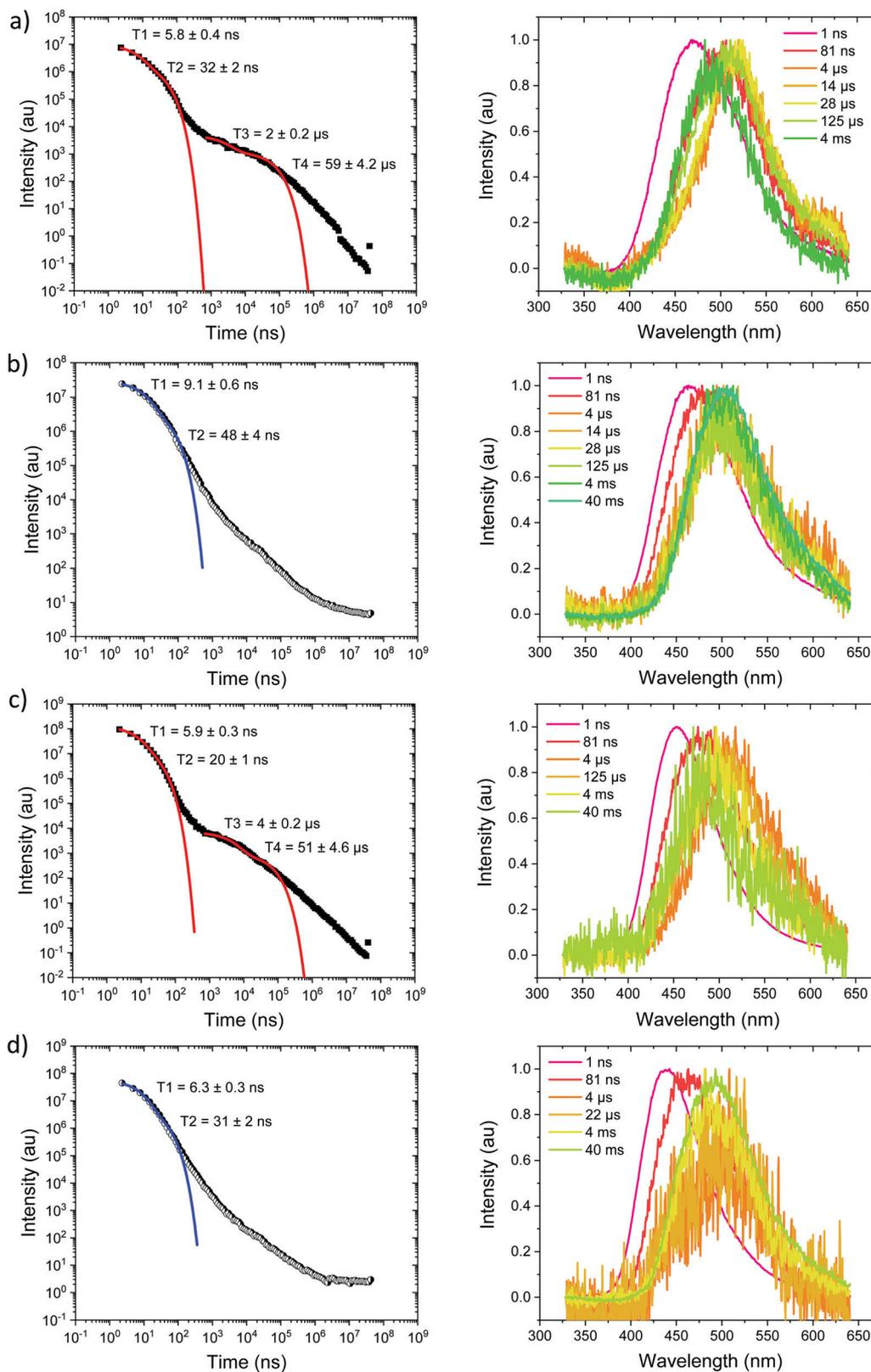
Fig. 7 Time-resolved spectrally integrated intensity decay (left) and representative time resolved spectra (right) of  $\text{Ph}_2\text{TRZCzPhCz}$ , (a) 300 K and (b) 80 K;  $\text{Ph}_3\text{TRZCzPhCz}$ , (c) 300 K and (d) 80 K in DPEPO host. Spectral times given in ns, and decay fitting data included in the decay plots.
