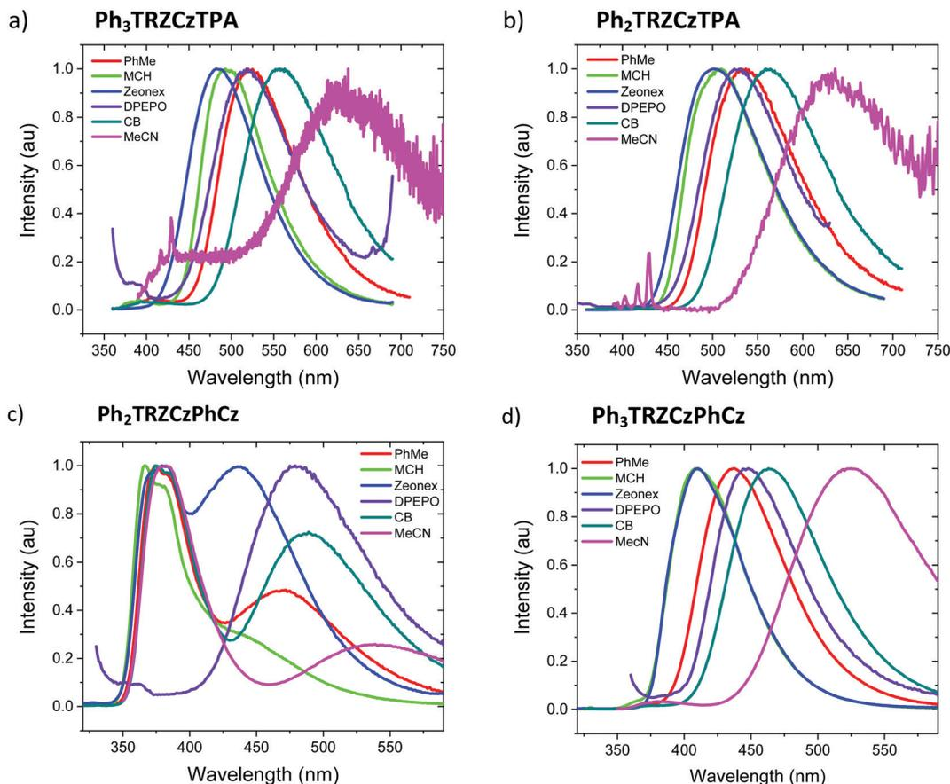
Fig. 3 Emission spectra of the compounds (a)  $\text{Ph}_3\text{TRZCzTPA}$ , (b)  $\text{Ph}_2\text{TRZCzTPA}$ , (c)  $\text{Ph}_2\text{TRZCzPhCz}$  and (d)  $\text{Ph}_3\text{TRZCzPhCz}$  in film and different solvents, methylcyclohexane (MCH), chlorobenzene (CB) and acetonitrile (MeCN).
