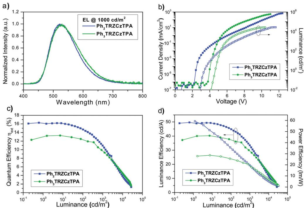
Fig. 9 (a) Normalized EL spectra at a luminance of  $10^3$   $\text{cd m}^{-2}$ ; (b) current density–luminance–voltage ( $J$ – $V$ – $L$ ) characteristics; (c) external quantum efficiency versus luminance, (d) luminance/power efficiency versus luminance for devices A and B.
