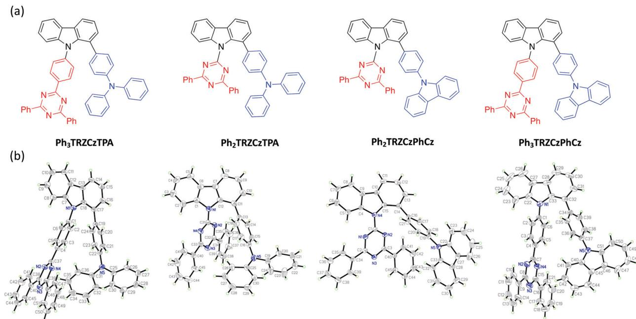
Fig. 1 The chemical structures (a) and X-ray structures (b) of **Ph<sub>3</sub>TRZCzTPA**, **Ph<sub>2</sub>TRZCzTPA**, **Ph<sub>2</sub>TRZCzPhCz** and **Ph<sub>3</sub>TRZCzPhCz**, thermal ellipsoids were drawn at a 50% probability level.
