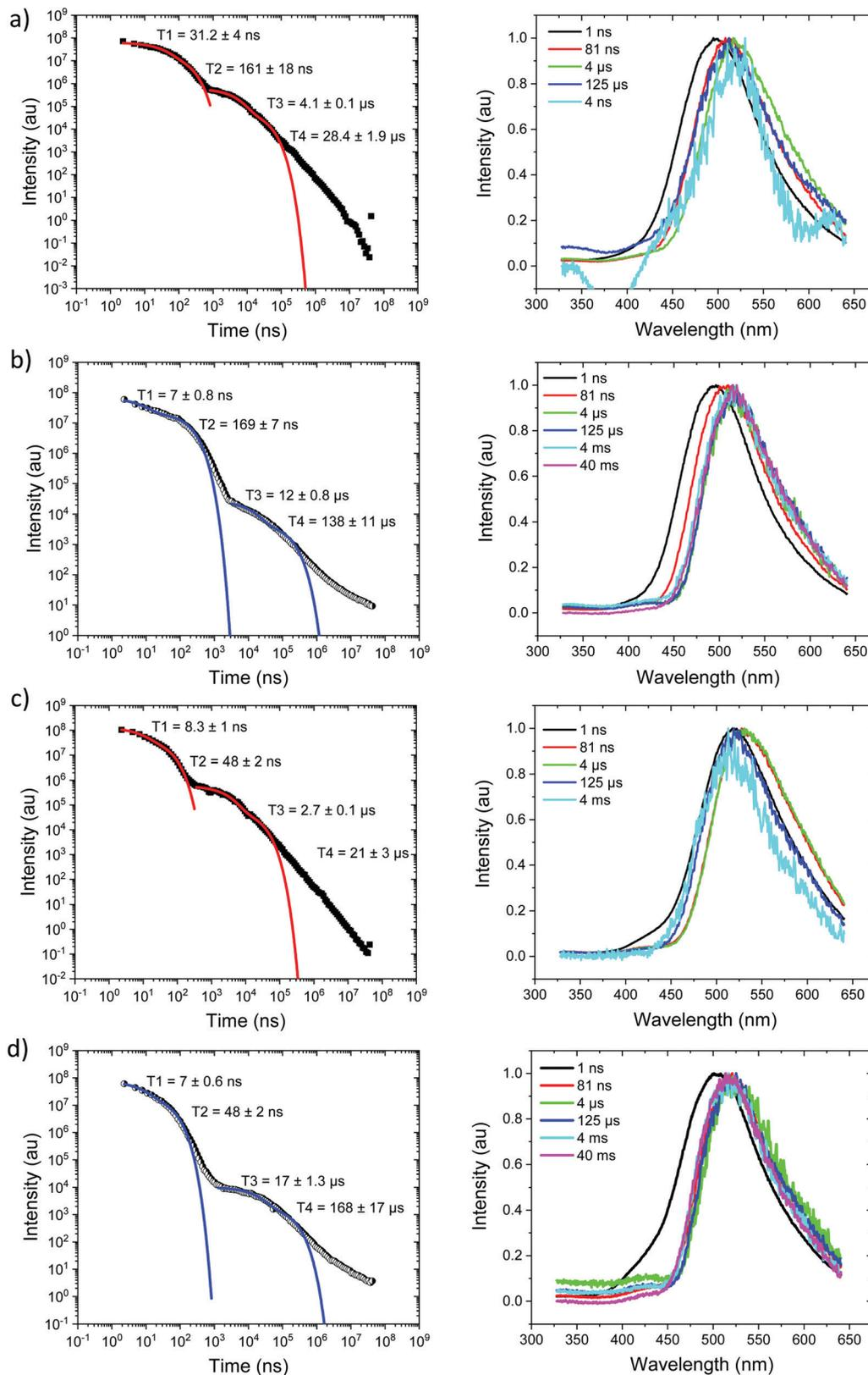
Fig. 6 Time-resolved spectrally integrated intensity decay (left) and representative time resolved spectra (right) of  $\text{Ph}_3\text{TRZCzTPA}$  (a) 300 K and (b) 80 K;  $\text{Ph}_2\text{TRZCzTPA}$  (c) 300 K and (d) 80 K in DPEPO host. Spectral times given in ns, and decay fitting data included in the decay plots.
