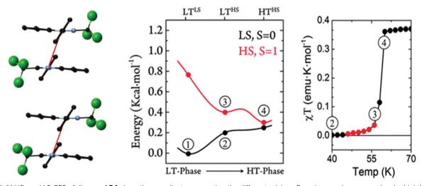
Fig. 13 (left) HS- and LS-PES of dimers of B4 along the coordinate connecting the different minima. Energies are given per molecule. (right) Magnetic susceptibility curve of **B4** around  $T_{1/2}$ . In red, we highlight the points with  $\chi T \neq 0$  before the jump. The key steps of the phase transition are numbered in both plots, as discussed in the main text. Reprinted/adapted with permission from ref. 176.
