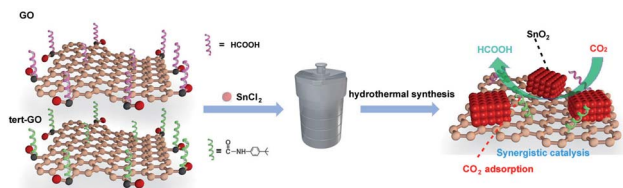
Fig. 1 Synthesis scheme of \text{SnO}_2/\text{GO} and \text{SnO}_2/\text{tert-GO} .
