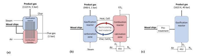
Fig. 2 Schematic representation of the gasification technologies considered in this work: (a) heat pipe reformer (HPR), (b) sorption enhanced reforming gasifier (oxySER) and (c) entrained flow gasifier (EF).
