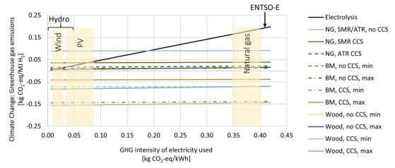
Fig. 15 Life cycle climate change impacts for  $H_2$  production *via* water electrolysis, reforming of natural gas (NG) or biomethane (BM), and gasification of wood. A similar figure has already been published in ref. 1 and has now been extended to include the wood gasification configurations. Results are shown in relation to the greenhouse gas intensity of the input electricity to the processes electrolysis, reforming, or gasification, respectively.
