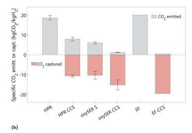
Fig. 6 (a) Comparison of the net efficiency (left y-axis, black dots and gray areas) and of the overall CO<sub>2</sub> capture rate (right y-axis, red diamonds and areas). (b) This figure shows the specific CO2 captured and emitted in each production chain. For the HPR and oxySER cases the bar corresponds to the base case, while the error bar highlights the variation due to the sensitivity analysis on different parameters and product gas composition.
