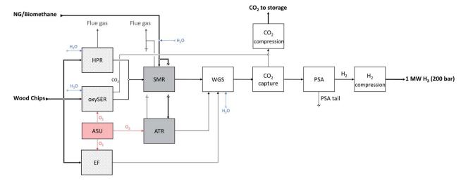
Fig. 1 Schematic representation of all hydrogen production pathways modelled and analysed in this work.
