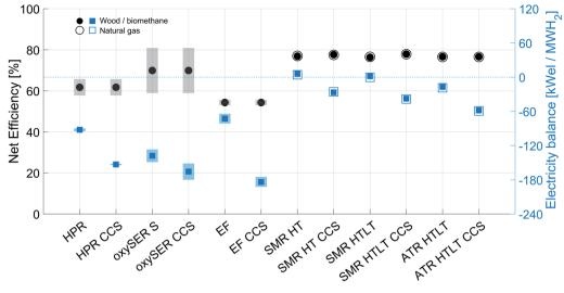
Fig. 8 Comparison of the net efficiency (black) and the electricity balance (light blue) between wood and natural gas/biomethane  $H_2$  chains. The light-blue dotted line illustrates the 0 value for the electricity balance: all cases that are below this threshold have to import electricity while the cases that are above have electricity in excess to be fed into the grid.
