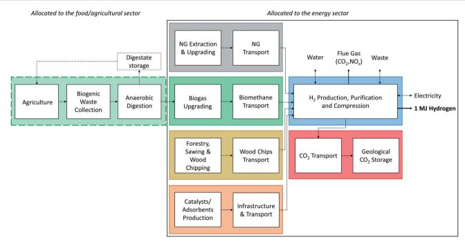
Fig. 4 System boundaries chosen for the LCA of H<sub>2</sub> production from natural gas (NG), biomethane, or wood as feedstock. The chain of the wet waste biomass down to the by-product biogas from treatment of the wet waste biomass in an anaerobic digestion plant is allocated to the food and agriculture sector. Extended from our previous work.<sup>1</sup>
