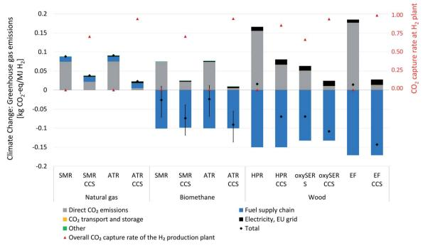
Fig. 9 Contribution of life cycle phases to the impacts on climate change from production of 1 MJ H<sub>2</sub> at 200 bar via selected technologies and system designs. The right y-axis shows the overall CO<sub>2</sub> capture rate at plant level. The category "Other" includes "Catalyst and Adsorbents", "Direct emissions from fuel combustion in furnace", "H2 production unit infrastructure", and "Water supply".
