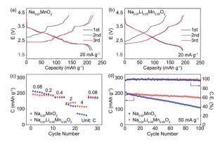
Fig. 6 Charge and discharge profiles of (a) P'2-Na $_{0.67}$ MnO $_2$  and (b) P'2-Na $_{0.67}$ Li $_{0.05}$ Mn $_{0.95}$ O $_2$  at 20 mA g $^{-1}$ . (c) Rate capability comparison of and P'2-Na $_{0.67}$ MnO $_2$  and P'2-Na $_{0.67}$ Li $_{0.05}$ Mn $_{0.95}$ O $_2$  at different rates. (d) Cycle performance of P'2-Na $_{0.67}$ MnO $_2$  and P'2-Na $_{0.67}$ Li $_{0.05}$ -Mn $_{0.95}$ O $_2$  at 50 mA g $^{-1}$ .
