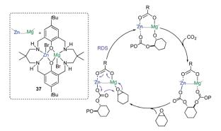
Fig. 10 Proposed mechanism for CO<sub>2</sub>/epoxide copolymerization by hetrobimetallic catalyst 37.
