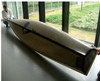
Fig. 2 Flax/PLA canoe manufactured during the NAVECOMAT project.
