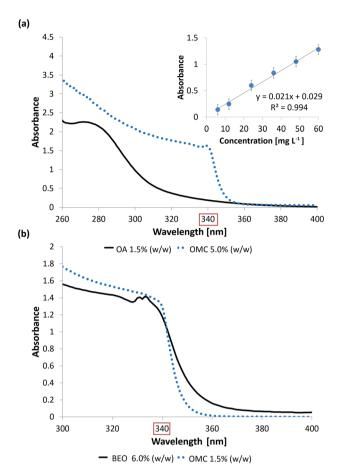
Fig. 2 (a) UV absorption spectra of a 1.5% (w/w) OA standard solution (black solid line) and a 5.0% (w/w) OMC standard solution (blue dotted line). The calibration curve for OMC at 340 nm and in the concentration range of 6.0-60.0 mg L $^{-1}$  is also shown. (b) UV absorption spectra of a 6.0% (w/w) BEO standard solution (black solid line) and a 1.5% (w/w) OMC standard solution (blue dotted line).
