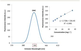
Fig. 3 Fluorescence spectrum corresponding to a standard solution of OMC (30 mg  $L^{-1}$ ). The characteristic maximum of signal at 390 nm and the calibration curve in the concentration range of 6.0–36.0 mg  $L^{-1}$  are shown. It is important to note that OA is not fluorescent around 390 nm.
