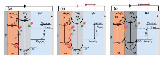
Fig. 1 Approximate energy band diagram and charge transfer mechanism of (a)  $Fe_2O_3-TiO_2$  photoanode without external applied anodic potential, (b)  $Fe_2O_3-TiO_2$  photoanode with external applied anodic potential and (c)  $Fe_2O_3-H:TiO_2$  photoanode with external applied anodic potential.
