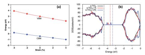
Fig. 4 (a) The calculated VBM and CBM of anatase using HSE06 under different biaxial strain. (b) The DOS of H doped a-TiO<sub>2</sub> compared with pure a-TiO<sub>2</sub>. The energy was aligned by the 1s state of O atom far away from the defect. The dashed line indicates the Fermi level of each system.
