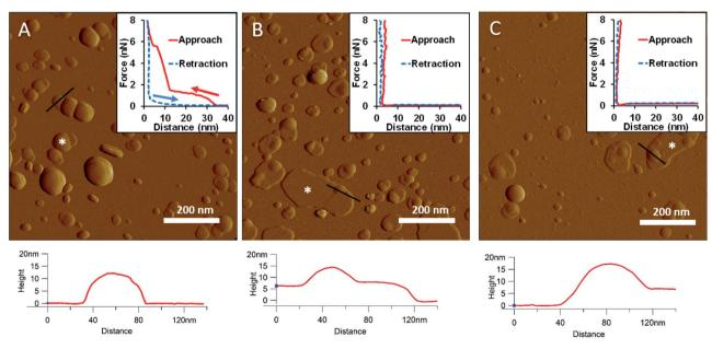
Fig. 2 Amplitude-contrast AFM image of LPS vesicles in the presence of  $10 \text{ mM Ca}^{2+}$ ; at  $20 \,^{\circ}\text{C}$  (A). The sample was warmed to  $50 \,^{\circ}\text{C}$  (B); and then cooled back to  $20 \,^{\circ}\text{C}$  (C). Insets: force–distance curves recorded while pressing LPS at the locations marked by the white star on each image. On the inset of A arrows indicate the direction of tip movement. Lower panels show height profiles taken along the black lines.
