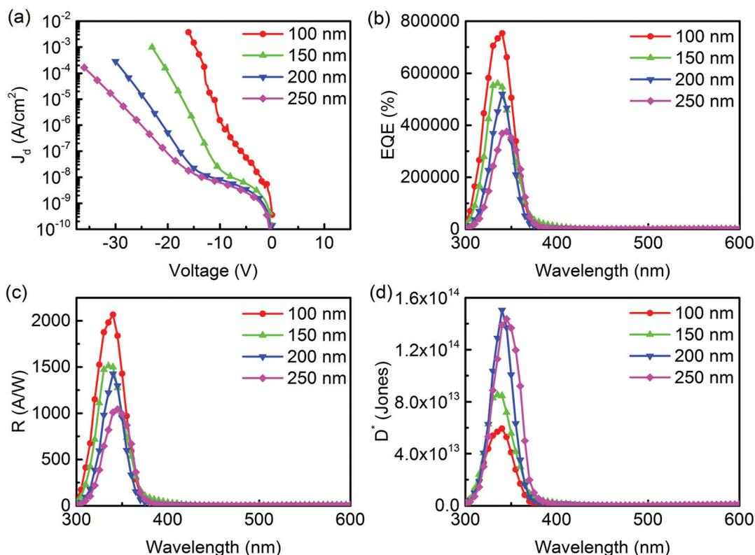
Fig. 4 (a)  $J_d$ , (b) EQE, (c)  $R$ , and (d)  $D^*$  characteristics of the fabricated UV PM-type OPDs with different active layer thicknesses. The device structure is ITO/TAPC: $C_{60}$ (50:1, 100 nm, 150 nm, 200 nm, 250 nm)/Al (100 nm).
