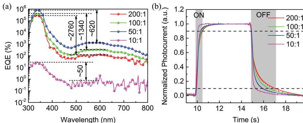
Fig. 6 (a) EQE and (b) transient photocurrent responses of the fabricated OPDs with different donor: acceptor doping ratios at  $-14$  V and 365 nm illumination. The pulse frequency is 0.1 Hz. The used device structure is ITO/TAPC:C<sub>60</sub>(200:1, 100:1, 50:1, 10:1, 80 nm)/Al.
