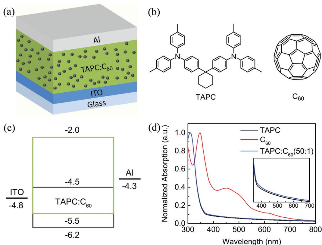
**Fig. 1** (a) Device structure diagram of the fabricated UV PM-type OPDs. (b) Chemical structures of the used organic materials. (c) Energy level diagram of the fabricated UV PM-type OPDs. (d) Normalized absorption spectra of TAPC,  $\text{C}_{60}$  and TAPC: $\text{C}_{60}$  blend films. Inset: Absorption spectra of TAPC and TAPC: $\text{C}_{60}$  (50 : 1, wt/wt) films in the wavelength range of 350–700 nm.
