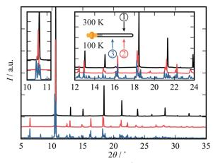
Fig. 3 Diffraction patterns ( $\lambda = 0.82484 \text{ Å}$ ) collected for a sample of Cd(CN)<sub>2</sub> at 300 K (black) and in the same position at 100 K (red) and at 100 K having been translated (blue = minimal prior exposure). The nature of the phase transition is clearly affected by irradiation prior to cooling.
