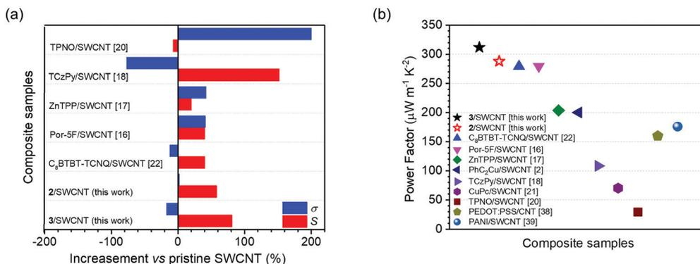
Fig. 4 (a) Increase of  $S$  and  $\sigma$  values of p-type thermoelectric composites made by SWCNT and organic small molecule semiconductors compared with pristine SWCNT. (b) A comparison of the PF values of p-type thermoelectric composites.
