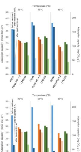
Fig. 20 Effect of propylene oxide modification of TEPA- and PEHA-based adsorbents on  $CO_2$  adsorption under 95%  $CO_2$  in 25, 55, and 85 °C for 3 h before and after treatment under air or  $N_2$  at 100 °C for 20 h. Comparison with LPEI25k/50S. Reproduced with permission from ref. 70. Copyright 2019, John Wiley and Sons.
