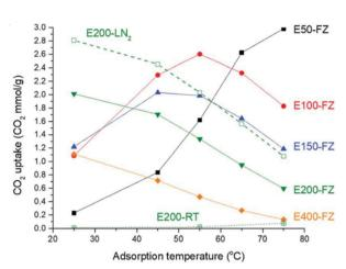
Fig. 11 Variation in  $CO_2$  capacity with temperature for different amine/cross-linker compositions. Adsorption under  $10\% CO_2$  for 3 hours. Reproduced from ref. 117 with permission from the Royal Society of Chemistry.
