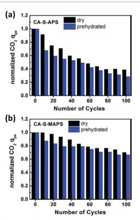
Fig. 24 Comparison of the cyclic CO<sub>2</sub> capacity of dry fibres and prehydrated fibres in 200 ppm  $SO_2$  in 10%  $CO_2/N_2$  at 35  $^{\circ}C$  of; (a) primary aminegrafted and; (b) secondary amine-grafted fibres. CO2 capacities normalised to adsorbents' initial  $CO_2$  capacity  $q_{pe,0}$  before exposure degradation. Reprinted from ref. 36 Copyright (2015), with permission from Elsevier.
