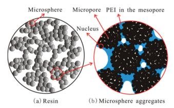
Fig. 14 Schematic diagram for PEI distribution in HP20. Reprinted with permission from ref. 28. Copyright (2013) American Chemical Society
