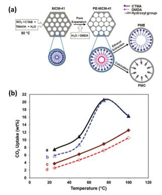
Fig. 12 (a) Schematic representation of the syntheses of PMC and PME. (b) CO<sub>2</sub> uptake *versus* temperature for (a) PME-PEI(55) after 180 min, (b) PME-PEI(55) after 30 min, (c) PMC-PEI(55) after 180 min, and (d) PMC-PEI(55) after 30 min of exposure to pure CO<sub>2</sub>. Adapted with permission from ref. 127. Copyright (2011) American Chemical Society.
