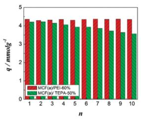
Fig. 17 CO<sub>2</sub> adsorption capacity of cyclic CO<sub>2</sub> adsorption-desorption of MCF(a)/PEI-60% and MCF(a)/TEPA-50%. Reprinted with permission from ref. 141. Copyright (2012) American Chemical Society
