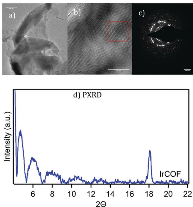
Fig. 7 (a) and (b) HRTEM images of IrCOF showing platelet structures, ordered multilayers, see ESI† Fig. S13 for enlargement of (b) and (c) a selected area of diffraction of the area in red box. See ESI,† Fig. S14–S19 for additional images including PtCOF & NiCOF including PXRD. (d) Thin-film PXRD of experimental IrCOF.
