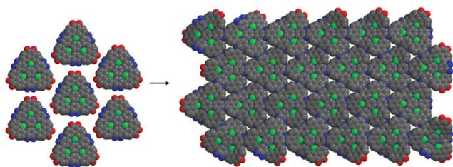
Fig. 1 Left: 3D space-filling models of seven monomers of **4** in a pre-polymerization configuration, gray = carbon, blue = nitrogen, red = oxygen, green represents either an empty pore or metal atom, hydrogens omitted. Right: 3D space-filling model of the resulting **COF**.
