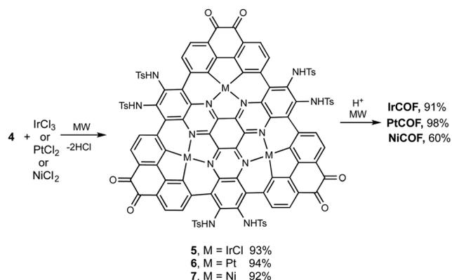
Scheme 2 Incorporation of metals into monomer **4** and formation of COFs. See Fig. 1 for COF drawings in which green represents metals.
