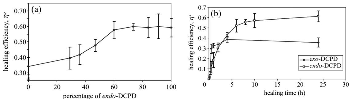
Fig. 18 Effect of DCPD on self-healing materials. (a) Effect of *exo/endo*-DCPD blends on healing efficiency. (b) Progress of healing efficiency for *endo*- and *exo*-DCPD with time [reproduced from ref. 189 with permission from the Royal Society of Chemistry].
