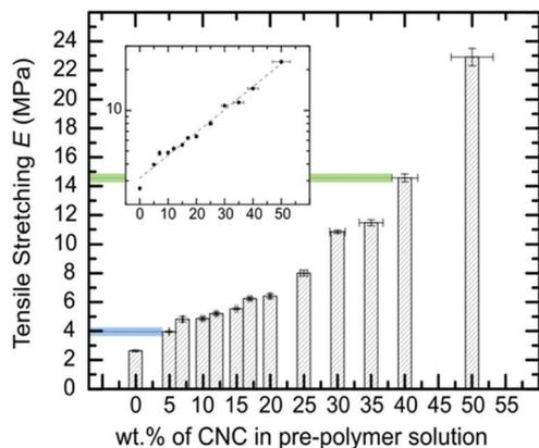
**Fig. 1** Evolution of the tensile Young's modulus of 6A-PCL/CNC composite films with the addition of CNCs (data measured by tensile stretching). The values in blue and green match reported tensile deformation values of brain and skin tissues, respectively. The inset shows the  $E$  in log10 scale, to emphasize the exponential dependency found with the addition of CNCs.
