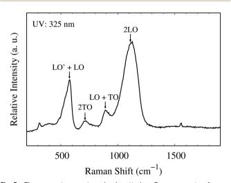
**Fig. 5** The room-temperature backscattering Raman spectra from a 325 nm excitation source. LO' + LO (430–635 cm $^{-1}$ ), 2TO (720 cm $^{-1}$ ), LO + TO (850–940 cm $^{-1}$ ) and 2LO (1120 cm $^{-1}$ ).
