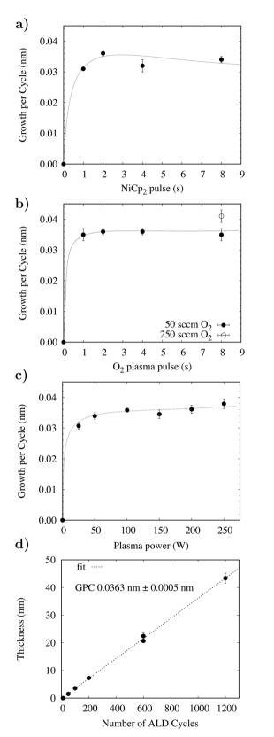
Fig. 2 Optimisation of the Ni(Cp)<sub>2</sub> PEALD process, all depositions completed at 250 °C. (a) Growth rate with respect to the Ni(Cp)<sub>2</sub> delivery pulse. (b) Growth rate vs. O<sub>2</sub> plasma pulse. (c) Growth rate as a function of plasma power. (d) Linearity of growth rate of NiO with respect to the number of ALD cycles.
