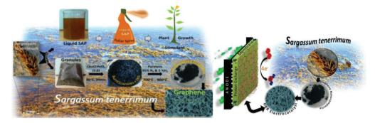
Fig. 12 Schematic showing the production of magnetite-functionalized graphene from Sargassum tenerrimum and scalable production method for Fe<sub>3</sub>O<sub>4</sub>/Fe-doped graphene nanosheets having electrocatalytic activity using DESs (reproduced from ref. 158 with permission from The Royal Society of Chemistry).
