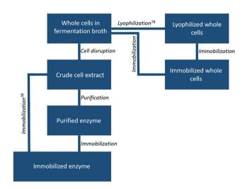
Fig. 5 Possible enzyme formulations and how they can be prepared from cultivated cells. Whole cells can be used directly as the catalyst, or be lyophilized or immobilized. Otherwise, cells can be disrupted to obtain cell free extract, which can be purified or (directly) immobilized.
