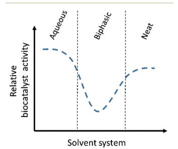
Fig. 2 Graphical representation of the activity of the transaminase on acetophenone and isopropylamine in different solvent systems from the example by Enzymaster. While the biocatalyst showed good activity in an aqueous buffer with cosolvent, only low conversions were observed when the pure substrate was added as a second phase. When the biocatalysts was introduced in a neat system however, an enhanced activity was determined again.
