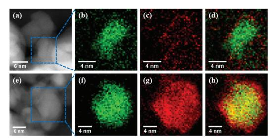
Fig. 7 Annular dark-field (ADF)-STEM images and corresponding EELS elemental maps of the spent  $Ni_3Fe_3/ZrO_2$  and  $Ni_3Fe_9/ZrO_2$  samples: (a) ADF-STEM image of  $Ni_3Fe_3/ZrO_2$ , (b-d) Ni (green), Fe (red), and mixed maps in  $Ni_3Fe_3/ZrO_2$ ; (e) ADF-STEM image of  $Ni_3Fe_9/ZrO_2$ , (f-h) Ni (green), Fe (red), and mixed maps in  $Ni_3Fe_9/ZrO_2$ .
