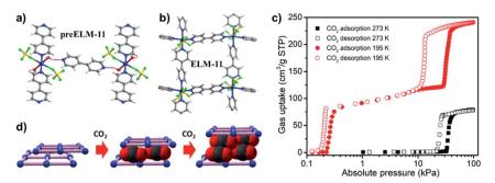
Fig. 16 The structures of (a) preELM-11 and (b) ELM-11; (c)  $\rm CO_2$  sorption isotherms of ELM-11 at 195 and 273 K; and (d) illustration of expansion/shrinkage of the adjacent layers in ELM-11. Figure (d) is reproduced from ref. 86 with permission; copyright: 2016, American Chemical Society.
