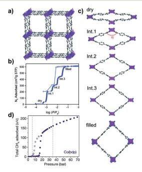
Fig. 14 (a) Crystal structure of as-synthesised Co(bdp); (b)  $N_2$  sorption isotherms of Co(bdp)-dry at 77 K; (c) phase transition during  $N_2$  sorption; and (d)  $CH_4$  sorption isotherms of Co(bdp)-dry at 298 K. Reproduced from ref. 74 and 102 with permission; copyrights: 2015, Springer Nature and 2010, American Chemical Society.
