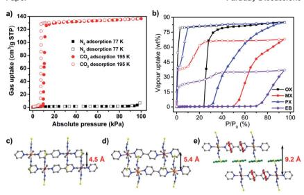
Fig. 17 (a and b)  $N_2$  (77 K),  $CO_2$  (195 K) and  $C_8$  vapour (298 K) sorption isotherms for sql-1-Co-NCS; (c-e) layer packing of nonporous,  $CO_2$ -loaded and xylene loaded phases of sql-1-Co-NCS, respectively.
