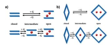
Fig. 4 Schematic illustration of the types of structural transformations in (a) 2D and (b) 3D switching CNs induced by sorbate/quest molecules (G, red balls). Transformation between closed and open phases typically results in a single-step type F-IV<sup>s</sup> isotherm (top). Transformation between closed, intermediate (partially open) and fully open phases generally leads to a type F-IV<sup>m</sup> isotherm (bottom).
