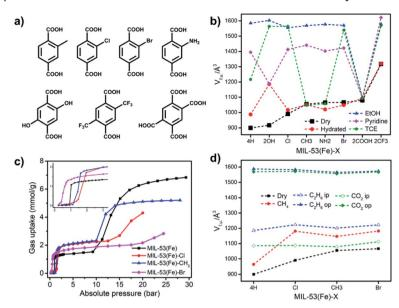
Fig. 8 (a) The functionalised bdc ligands used to synthesise MIL-53(Fe)-X variants; (b) and (d) volume per formula unit ( $V_{\rm fu}$ ) of MIL-53(Fe)-X variants under different conditions, 4H = MIL-53(Fe); (c) C<sub>2</sub>H<sub>6</sub> sorption isotherms of MIL-53(Fe)-X at 303 K.
