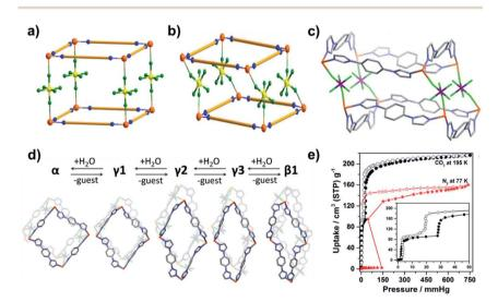
Fig. 12 Schematic diagrams of (a) traditional SIFSIX-n-M networks with trans-bridging SIFSIX pillars and (b) SIFSIX-23-Cu with cis-bridging SIFSIX pillars; (c) coordination mode and geometry in SIFSIX-23-Cu; (d) reversible structural transformations in SIFSIX-23-Cu; (e)  $N_2$  (77 K) and  $CO_2$  (195 K) sorption isotherms of SIFSIX-23-Cu. Reproduced from ref. 151 with permission; copyright: 2020, American Chemical Society.
