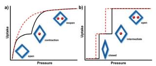
Fig. 6 Schematic illustrations of the sorption isotherm types reported for the MIL-53(M) family. (a) Type F-I isotherms with open to less open to open transformations as observed in MIL-53(Cr, Al); (b) type F-IV<sup>m</sup> isotherm with closed to open to more open transformations as seen for MIL-53(Fe, Sc). Black solid line: adsorption curve; red dash line: desorption curve.
