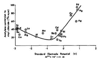
Fig. 17 Correlation of the activity of carbon-supported metal chloride catalysts for acetylene hydrochlorination. Reproduced with permission from ref. 53.
