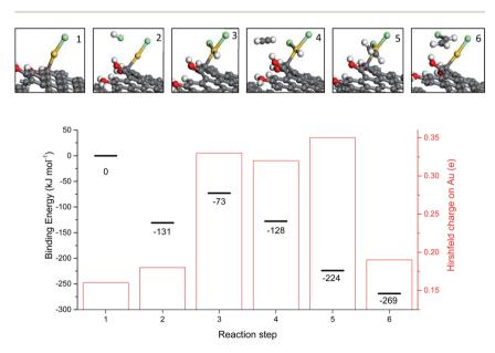
Fig. 19 Mechanism for the transformation of AuCl to AuCl<sub>2</sub>H and the formation of vinyl chloride, reproducing AuCl. Key: Au atoms (gold), Cl atoms (green), H atoms (white), C atoms (grey) and O atoms (red). Energies are referenced to the geometry optimized configuration of AuCl on the carbon support and gas phase acetylene and HCl. Binding energies for each energy minimum and the Hirshfeld charge on each Au atom are shown for each step. Reproduced with permission from ref. 2.
