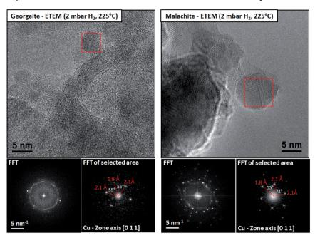
Fig. 1 The microstructures of the reduced georgeite and malachite precursors characterized by ETEM in 2 mbar  $H_2$  at 225  $^{\circ}$ C. Both samples reveal distinct Cu nanoparticles distributed on ZnO as confirmed by FFT analysis. The reduced malachite sample reveals in general larger Cu nanoparticles compared to the georgeite sample. Reproduced with permission from ref. 7.
