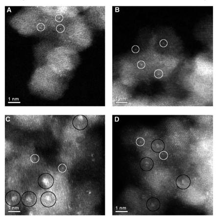
Fig. 12 High-magnification aberration-corrected STEM-HAADF images of (A and B) the inactive and (C and D) the active  $Au/FeO_x$  catalysts acquired with AC-STEM. The white circles indicate the presence of individual Au atoms, whereas the black circles indicate sub-nanometer Au clusters consisting of only a few atoms. Reproduced with permission from ref. 49.
