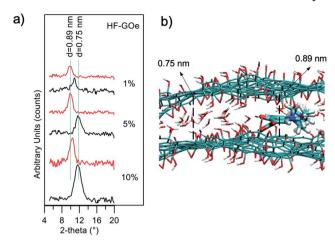
Fig. 11 (a) XRD patterns of HF-GOe fibers before (black) and after (red) filtration of organic microcontaminants. Two vertical lines as references are at angles corresponding to 0.89 nm and 0.75 nm. (b) GO bilayers after ofloxacin intercalation.
