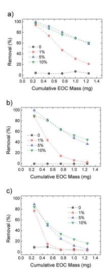
Fig. 9 Removal efficiency for Ciproflox (a), OFLOX (b) and RhB (c) for PES and increasing GO loading in HF-GOi. The cumulative initial mass is obtained with fixed concentration (5 mg  $L^{-1}$ ) and flow (15 mL min $^{-1}$ ). Details are reported in Fig. S10. The curves for HF-GOe filters are shown in Fig. S11, ESI.†
