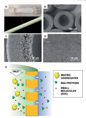
Fig. 1 (a) Versatile PES® hollow fiber filtration cartridge (lab. scale prototype 10 cm length (Plasmart 25, Medica)) and single fiber. In the cartridge the edges of the fiber capillaries are sealed by an epoxy resin. (b) Fibers, (c) cross-section, (d) detail of the outer wall pores. (e) Cartoon of filtration through the cartridge (in–out).
