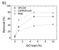
Fig. 8 Removal efficiency for OFLOX, Ciproflox and RhB vs. GO loading for (a) HF-GOe and (b) HF-GOi. The concentration (5 mg  $L^{-1}$ ), flow (15 mL min $^{-1}$ ) and fluxed volume (250 mL) of the contaminant solutions were the same for all tests. Filtration was performed by flowing water firstly passing through the GO layer, *i.e.* in–out for inner coated fibers and out–in for outer coated fibers.
