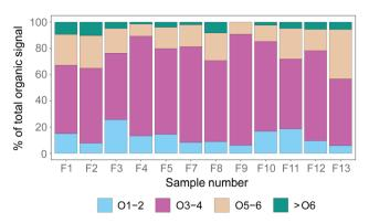
Fig. 7 Percentage of the sample signal from organic compounds including 1–2 oxygen atoms (O1–2), 3–4 (O3–4), 5–6 (O5–6) and more than 6 oxygen atoms (>O6).
