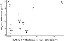
Fig. 4 Relationship between (a) total signal from organic compounds of each FIGAERO-CIMS sample and organic mass sampled by AMS aggregated to the filter sampling periods, (b) total signal of each FIGAERO-CIMS aerosol sample and the integrated particle mass of submicron aerosol aggregated to the filter sampling periods. F1–F13 are the sample numbers.
