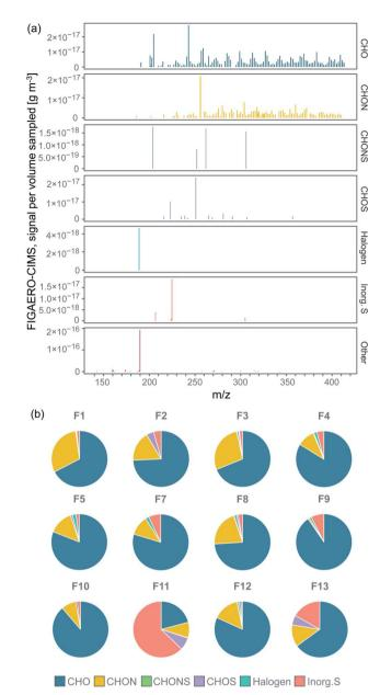
Fig. 2 (a) FIGAERO-CIMS high resolution mass spectrum of the sample median signal separated by compound category, showing where in the spectrum molecules of the different categories were found, (b) pie charts of the relative contribution to the total signal intensity (sampled mass per sampled volume) of the compound categories in each individual filter (the category *Other* not included). Percentages of the pie charts are listed in Table S3.†
