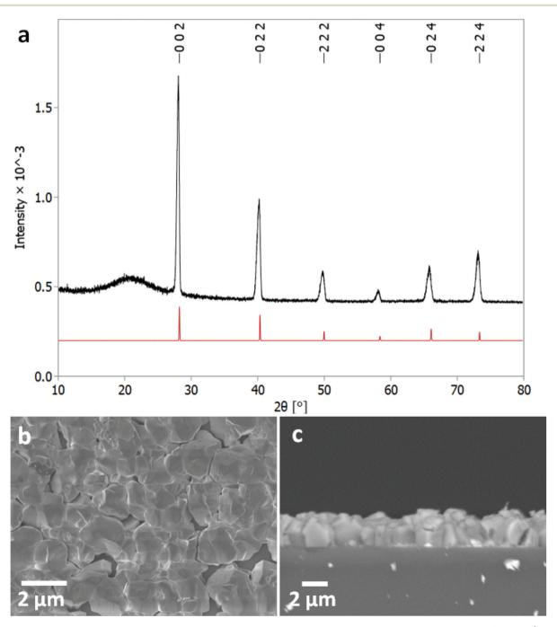
Fig. 2 (a) Grazing incidence XRD pattern for SnTe thin film (thickness  $\sim 2 \mu m$ ) with XRD pattern for bulk cubic SnTe ( $Fm\bar{3}m$ ) (red). The broad feature observed around 21° is due to the fused silica substrate beneath the SnTe film. Top down SEM (b) and cross-sectional SEM (c) of a SnTe film.
