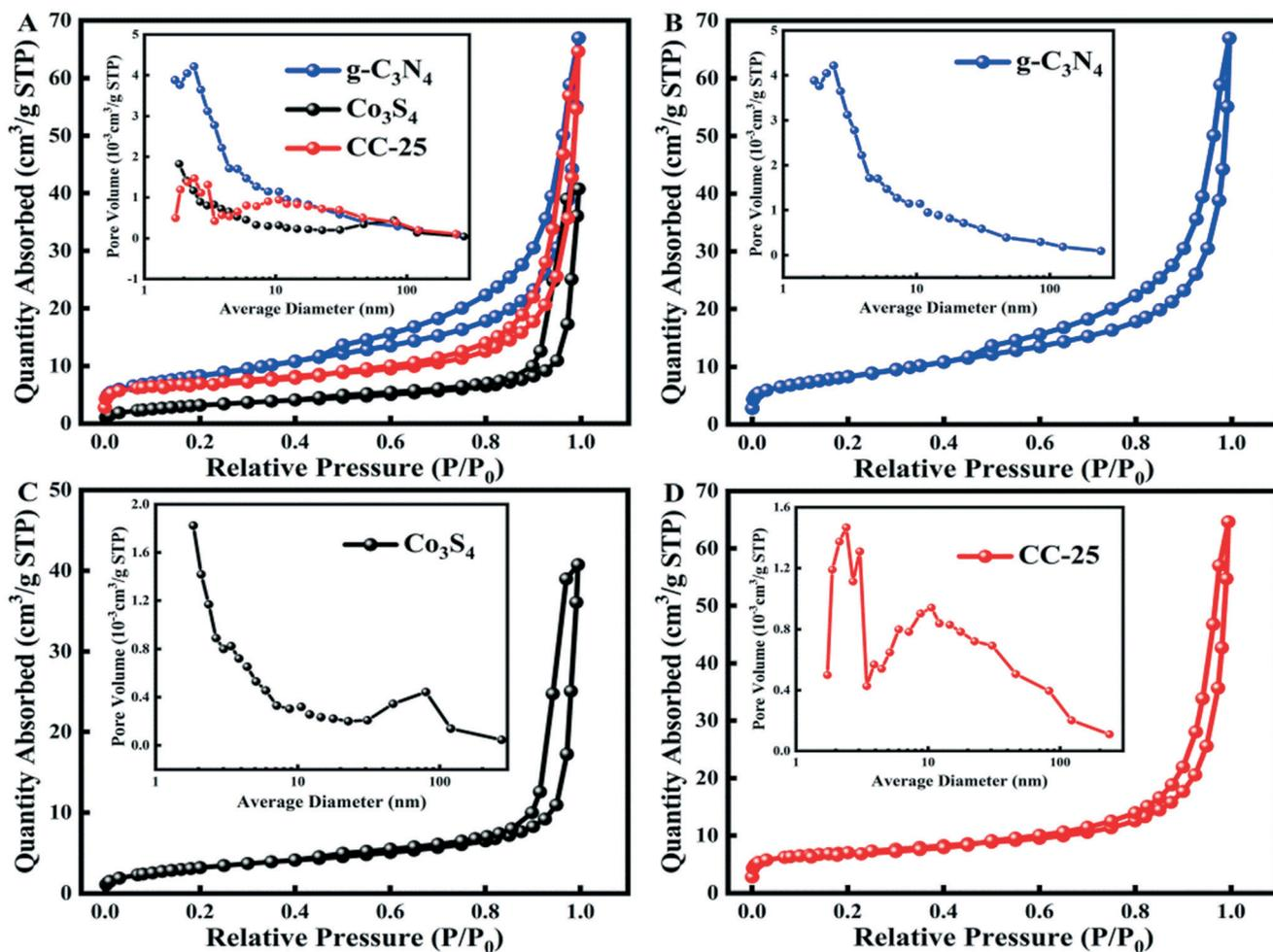
Fig. 4 (A) N<sub>2</sub> adsorption–desorption isotherms for g-C<sub>3</sub>N<sub>4</sub> tubes, Co<sub>3</sub>S<sub>4</sub>, and CC-25, and corresponding pore size distribution curves (inset). (B)–(D) N<sub>2</sub> adsorption–desorption isotherms for g-C<sub>3</sub>N<sub>4</sub> tubes, Co<sub>3</sub>S<sub>4</sub>, and CC-25, and corresponding pore size distribution curves (inset).
