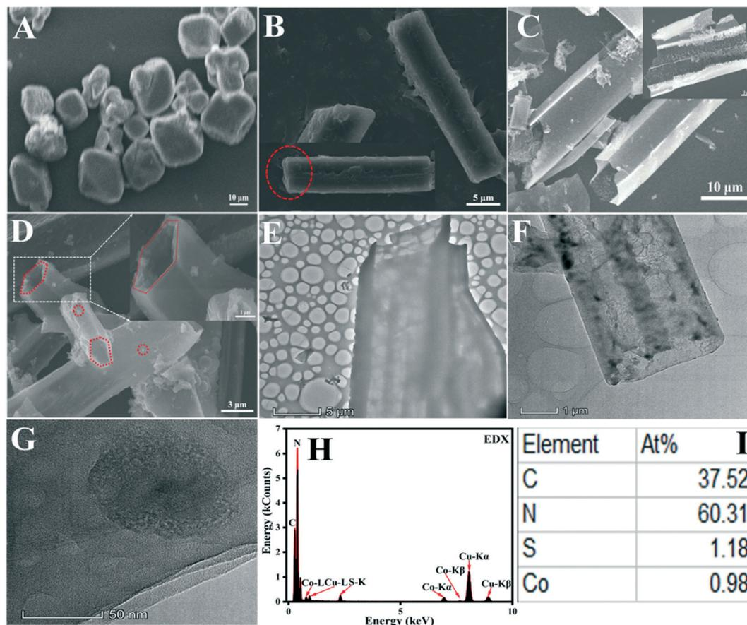
**Fig. 2** SEM images of (A) melamine raw material, (B) supramolecular precursor prepared by the hydrothermal method with melamine as the raw material, (C)  $g-C_3N_4$  tubes, (D) CC-25. TEM images of (E)  $g-C_3N_4$  tubes and (F) CC-25. HRTEM image of (G) CC-25. (H) EDX image of CC-25. (I) The atomic fractions of C, N, S, and Co.
