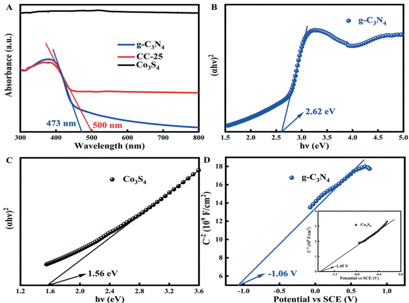
Fig. 8 (A) UV-vis diffuse reflectance spectra of g-C<sub>3</sub>N<sub>4</sub>, Co<sub>3</sub>S<sub>4</sub>, and CC-25. The corresponding plots of  $(\alpha h\nu)^2$  versus  $h\nu$  of (B) g-C<sub>3</sub>N<sub>4</sub> tubes and (C) Co<sub>3</sub>S<sub>4</sub>. (D) Mott-Schottky curves of g-C<sub>3</sub>N<sub>4</sub> and Co<sub>3</sub>S<sub>4</sub> (inset curve).
