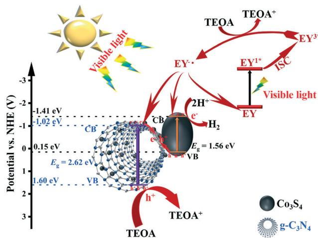
Fig. 9 Proposed mechanism for enhanced photocatalytic H<sub>2</sub> evolution under visible light irradiation.
