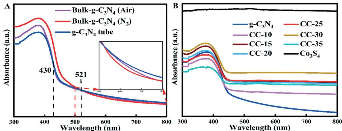
Fig. 5 UV-vis diffuse reflectance spectra of (A) g-C<sub>3</sub>N<sub>4</sub> (prepared under different conditions), (B) g-C<sub>3</sub>N<sub>4</sub> tubes, Co<sub>3</sub>S<sub>4</sub>, and CC-x (x = 10, 15, 20, 25, 30, 35).
