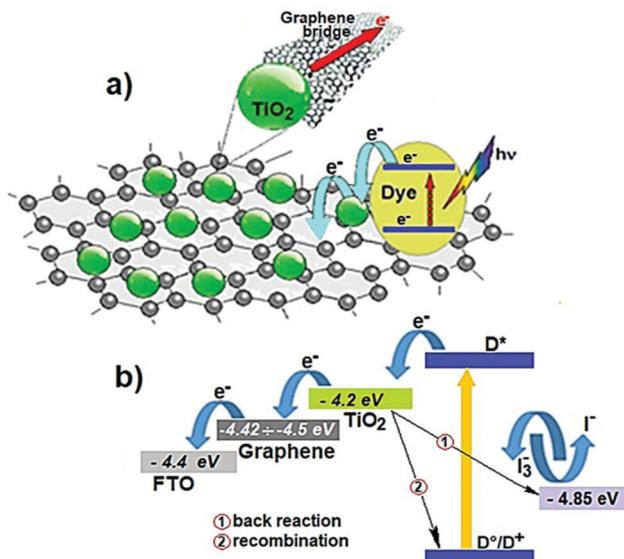
Fig. 11 (a) Schematic of light capture and electron transfer pathway from TiO<sub>2</sub> to the FTO, in TiO<sub>2</sub>/graphene-based DSSC photoanodes. (b) Schematic of the electron cascade route in DSSC using TiO<sub>2</sub>/graphene-based photoanodes.
