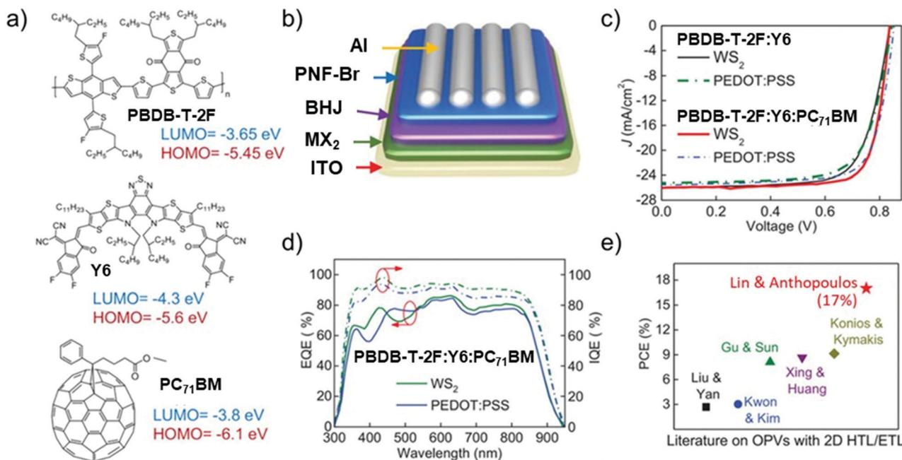
**Fig. 10** (a) Chemical structure of PBDB-T-2F, Y6, and PC<sub>71</sub>BM and the corresponding LUMO and HOMO energies. (b) Schematic of the standard OSC architectures employed. (c) *J*-*V* curves of OSCs based on PBDB-T-2F:Y6 and PBDB-T-2F:Y6:PC<sub>71</sub>BM with different HTLs. (d) EQE curves of OSCs based on a PBDB-T-2F:Y6:PC<sub>71</sub>BM active layer for different HTLs. (e) A comparison of the performances of previously reported OSCs with 2D material interfaces. Adapted from ref. 633.
