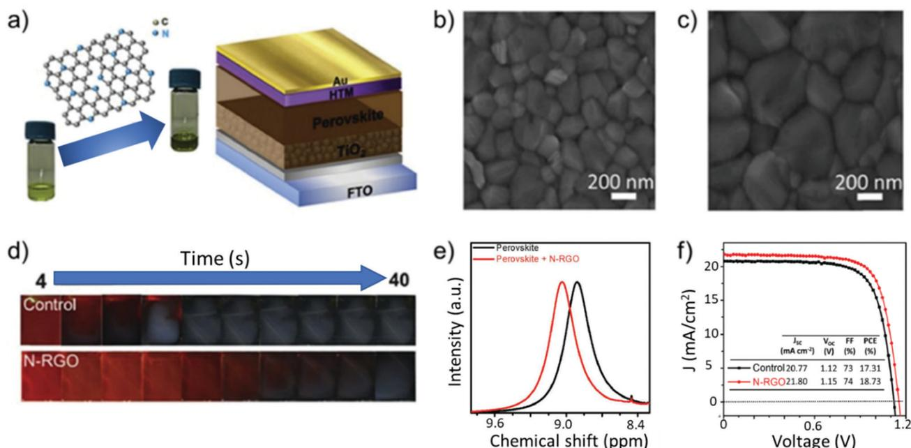
Fig. 21 (a) Schematic showing the N-RGO-doped perovskite solution and PSC with a structure of FTO/TiO<sub>2</sub>/N-RGO/perovskite/spiro-OMeTAD/Au. (b and c) SEM images of perovskite films before and after the incorporation of N-RGO. (d) Photographs of perovskite films during the annealing process at 100 °C. (e) <sup>1</sup>H NMR spectra of perovskite and N-RGO/perovskite solution. (f) *J*-*V* characteristics of the control device and N-RGO-incorporated device. Adapted from ref. 1134.
