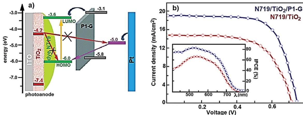
Fig. 13 (a) Schematic of the energy-level diagram and electron transfer process in P1-graphene-based DSSCs. (b)  $J$ - $V$  curves and IPCE spectra for DSSCs with and without a P1-G layer. Adapted with data from ref. 769.
