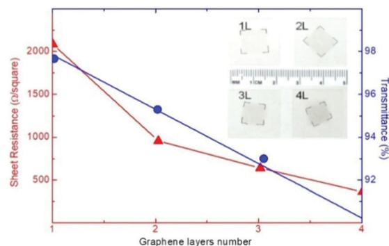
Fig. 4 Sheet resistance ( $R_s$ ) and transmittance ( $T_r$ ) of a graphene (film) as a function of the number of stacked graphene layers. Adapted from ref. 169, Copyright 2008, American Chemical Society.
