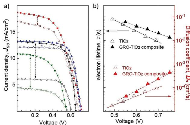
Fig. 14 (a) Typical  $J$ - $V$  curves of DSSCs based on different GRM-based photoactive layers (line and full symbols) compared to those of the corresponding traditional  $TiO_2$ -based photoelectrode. (b) Electron diffusion coefficient ( $D_n$ ) and lifetime ( $\tau$ ) dependence on the applied voltage for DSSCs based on  $TiO_2$  photoactive layers with and without GRMs. Adapted from ref. 741,742,758,759.
