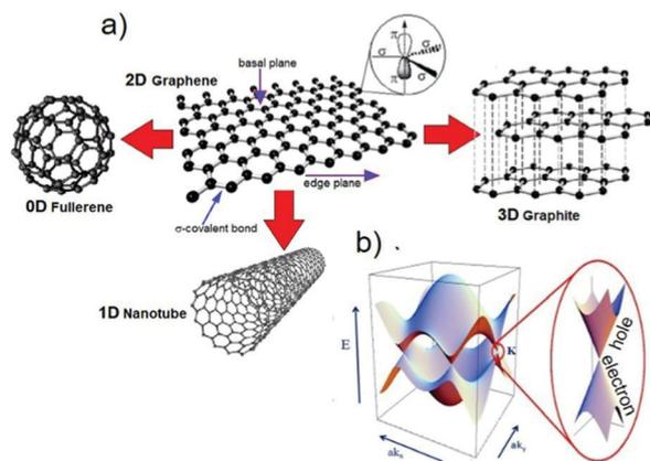
Fig. 3 (a) Schematic of the honeycomb graphene network as formed by C atoms and bonded  $\sigma$  bonds perpendicular to  $\pi$  orbitals. The other graphene-derived allotropes of C are also shown. Adapted from ref. 139 and 140. (b) Band structure in the honeycomb lattice. In the enlarged picture, the energy bands close to one of the Dirac points are also sketched. Adapted from ref. 141.
